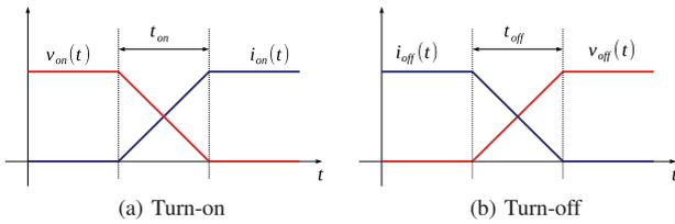
Figure 1: IGBT switching voltage and current approximation for power losses estimation
