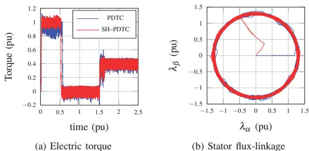
Figure 2: PDTC and SH-PDTC simulation results
