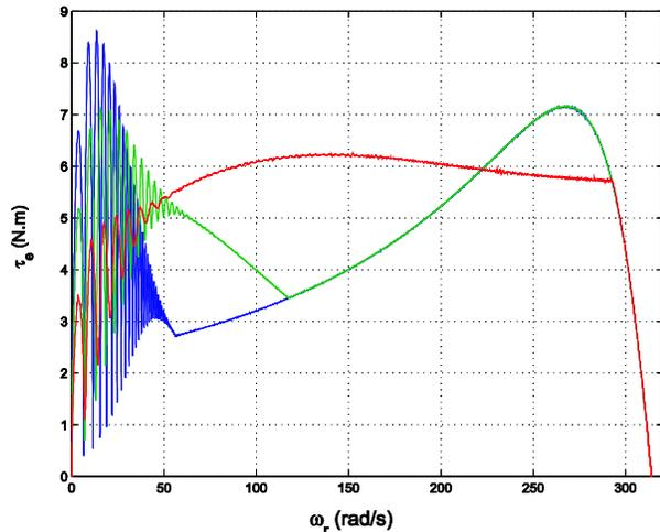
Fig. 3.- Example of a simulated torque under open loop V/f control for three different values of ramp-up frequency at start-up.
