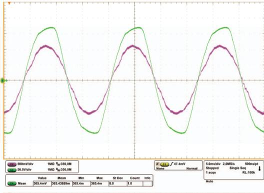
Figure 13: Experimental grid voltage and current with dead-times compensation when  $\hat{v}_g$  is used as feedforward signal.
