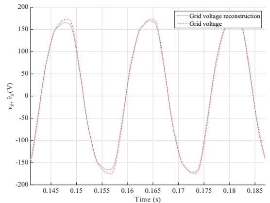
Figure 11: Measured grid voltage ( $v_g$ ) and its reconstructed version ( $\hat{v}_g$ ).
