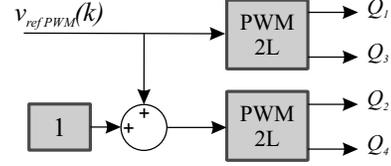
Figure 5: Pulse width modulator for the 3L-NPC.
