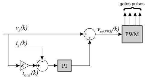
Figure 1: Proportional-integrative controller with feedforward of grid voltage.
