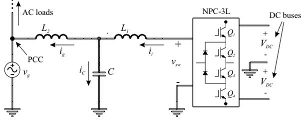
Figure 3: One-phase three-level neutral point clamped grid connected inverter.
