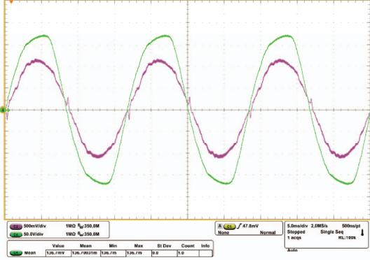
Figure 12: Experimental grid voltage and current without dead-times compensation when  $v_g$  is used as feedforward signal.
