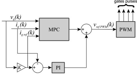
Figure 2: Hybrid control scheme with MPC and PI actions.
