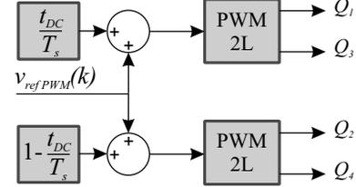
Figure 6: Pulse width modulator for the 3L-NPC with compensation of dead-times effect.
