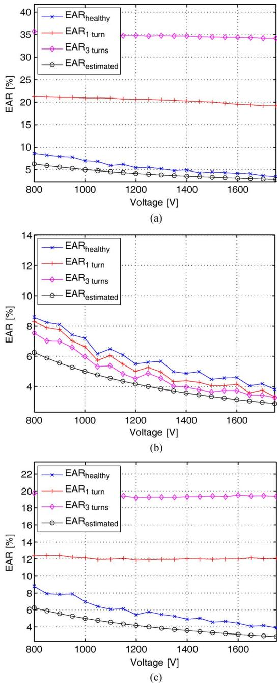
Fig. 8.  $EAR$  for the surge test applied to a healthy motor and a motor with one shorted turn and three shorted turns, respectively. (a)  $EAR$  obtained for an offline surge test. (b)  $EAR$  obtained for a surge test in the online configuration with 250- $\mu$ H supply inductance. (c)  $EAR$  obtained for a surge test in the online configuration with 9-mH supply inductance.
