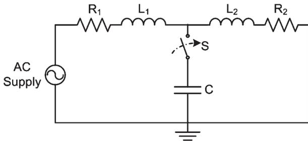
Fig. 3. Single-phase equivalent circuit of the online surge test.
