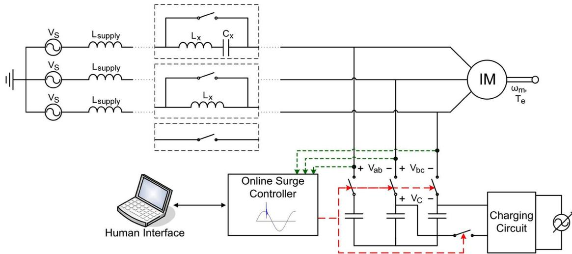
Fig. 2. Basic online surge schematic with additional supply impedance.
