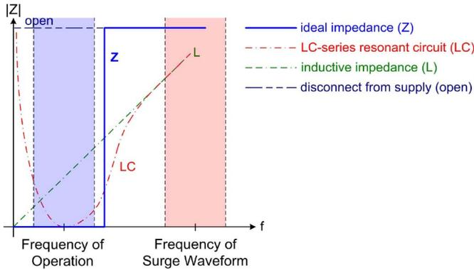
Fig. 4. Frequency characteristics of supply impedances suggested to separate the motor from the supply.
