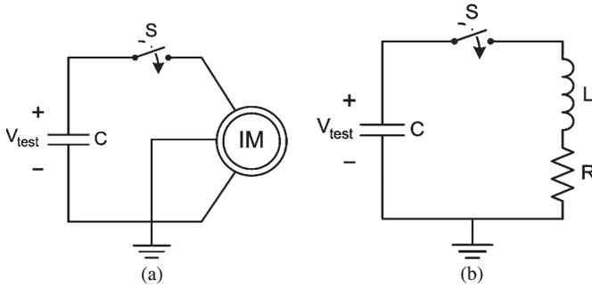
Fig. 1. Offline surge test schematic. (a) Surge test setup. (b) Equivalent circuit for the surge test.
