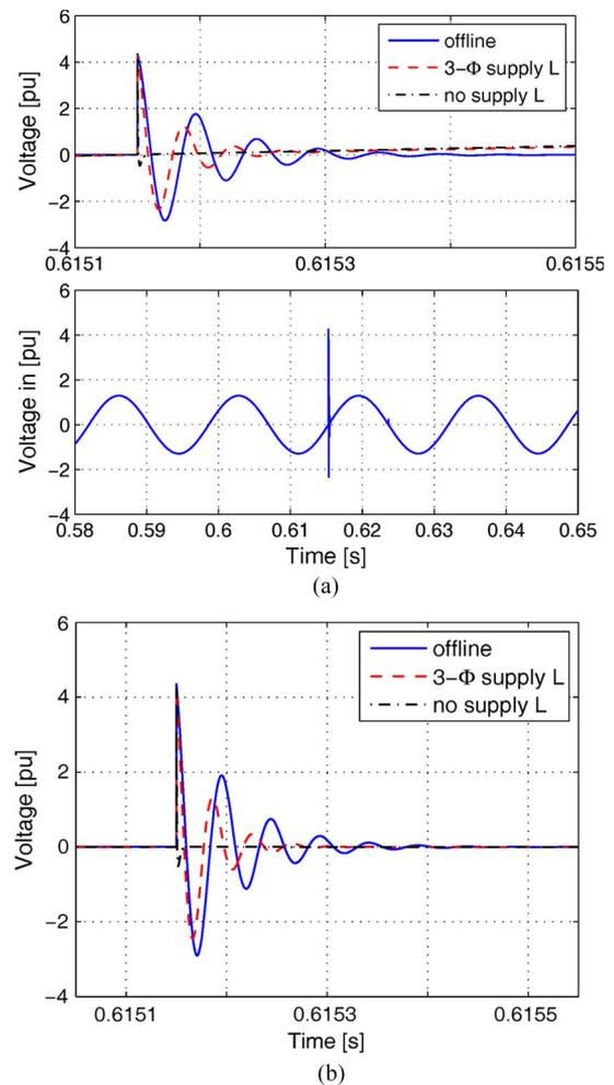
Fig. 6. Simulation results for the online surge test with an additional supply inductance in all three phases. (a) Online surge waveform for the additional supply inductance in all three phases compared to the offline waveform and the online waveform without additional supply impedance. (b) Online surge waveform for the additional supply inductance in all three phases with fundamental removed.
