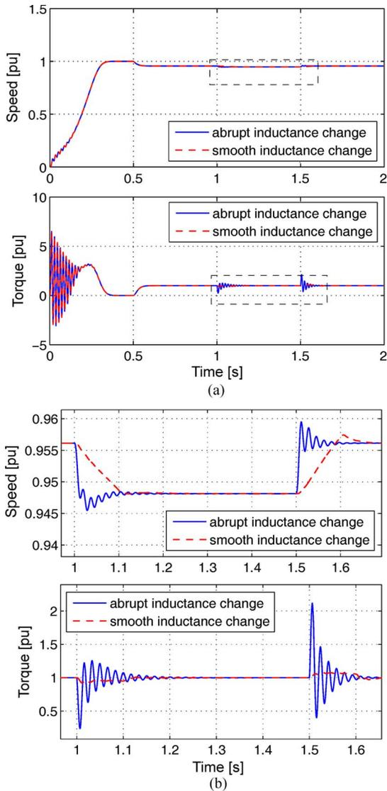
Fig. 5. Simulation results for the abrupt and smooth inductance changes of the additional supply inductor. (a) Torque and speed transients for the abrupt and smooth inductance changes. (b) Close-up of (a).
