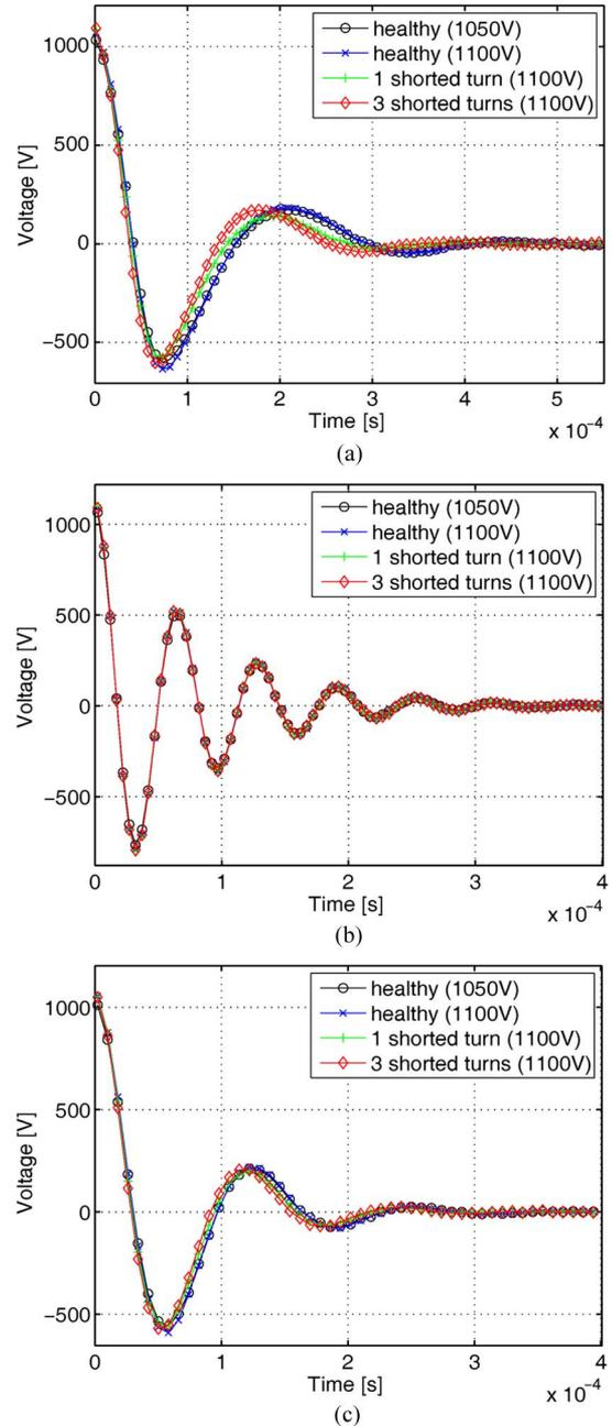
Fig. 7. Experimental results for a surge test applied to a healthy motor and a motor with one shorted turn and three shorted turns, respectively. (a) Offline surge test. (b) Surge test in the online configuration with 250- $\mu$ H supply inductance. (c) Surge test in the online configuration with 9-mH supply inductance.
