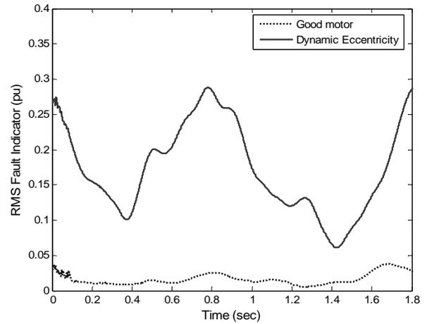
Figure 12. RMS fault indicator for fault discrimination (dynamic eccentricity).
