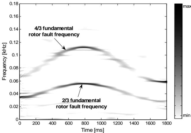
Figure 11. SPWVD of BLDC motor with dynamic eccentricity (5 Hz sinusoidal speed reference).
