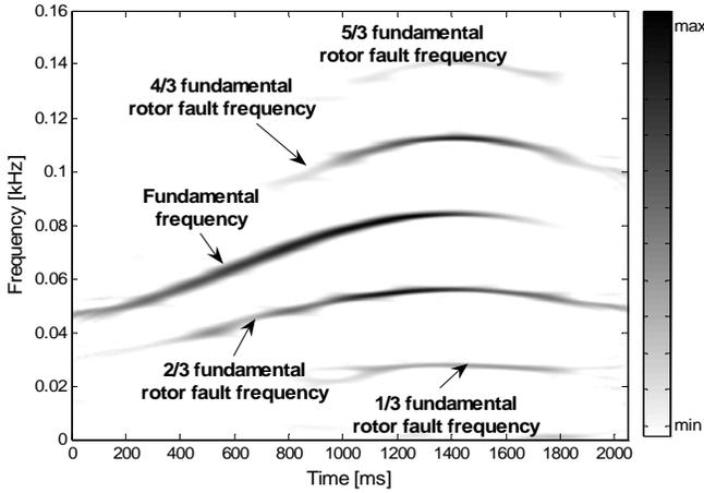
Figure 9. SPWVD of mechanically unbalanced BLDC motor (3 Hz sinusoidal speed reference).
