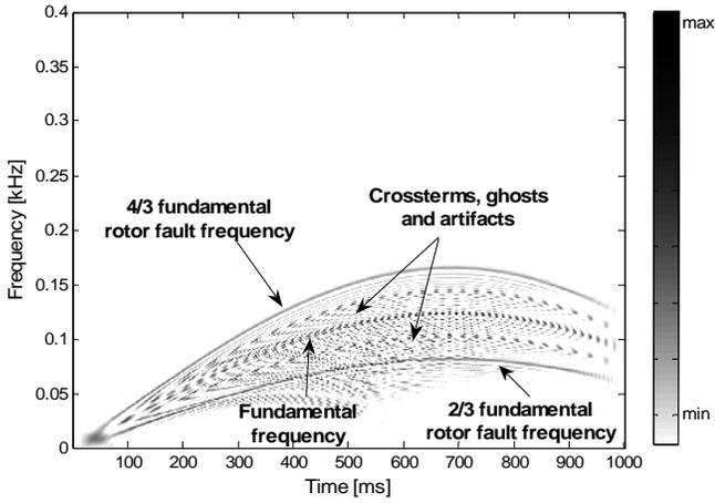
Figure 3. WVD of a simulated BLDCM rotor fault using a hypothetical test signal  $i_d$ .
