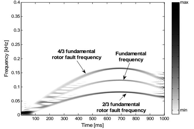
Figure 5. SPWVD of a simulated BLDCM rotor fault using a hypothetical test signal  $i_d$ .
