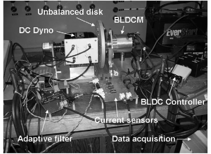
Figure 8. Experimental arrangement to implement BLDC rotor faults.
