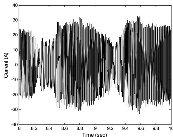
Figure 1. Non-stationary stator current in a BLDC motor.
