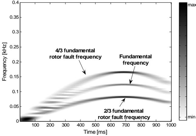
Figure 2. STFT of a simulated BLDCM rotor fault using a hypothetical test signal  $i_d$ .
