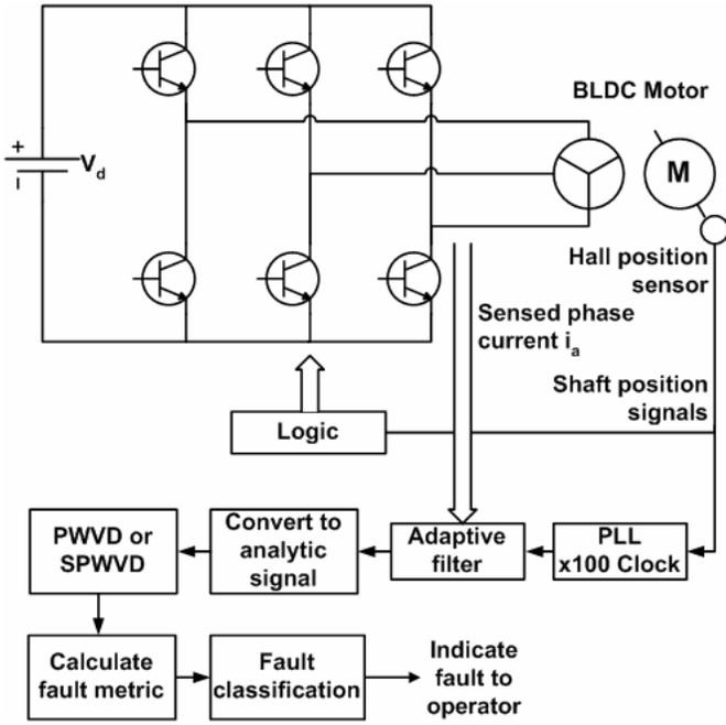
Figure 6. SPWVD / PWVD based BLDC rotor fault detection.
