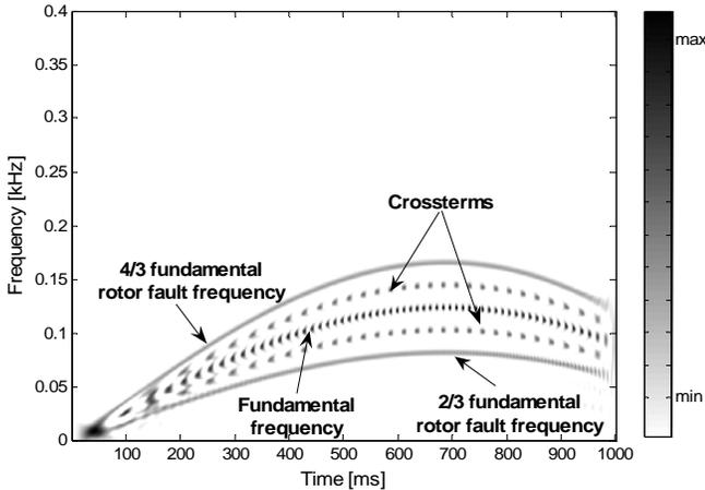
Figure 4. PWVD of a simulated BLDCM rotor fault using a hypothetical test signal  $i_d$ .
