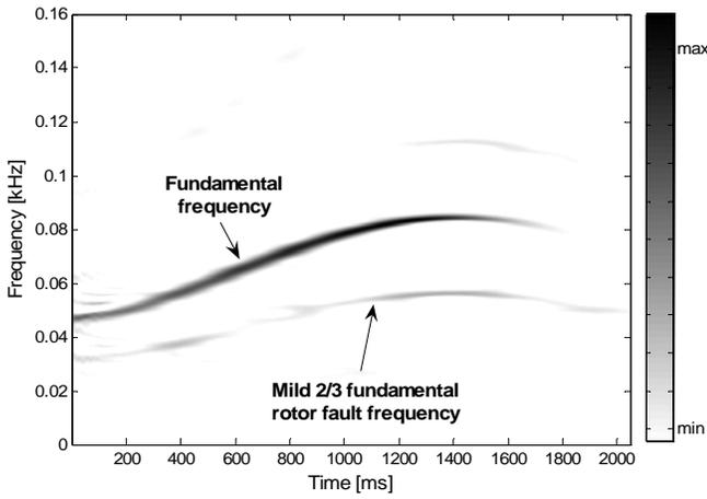
Figure 10. SPWVD of mechanically balanced BLDC motor (3 Hz sinusoidal speed reference).
