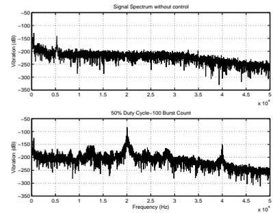
FIGURE 3: Vibration spectrum with 50% duty cycle and 100 cycle burst count.
