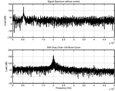
FIGURE 2: Dynamic Force spectrum with 50% duty cycle and 100 cycle burst count.
