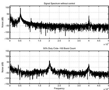
FIGURE 1: Noise spectrum with 50% duty cycle and 100 cycle burst count.
