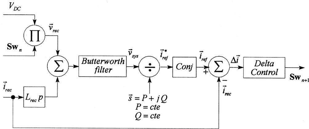
Fig. 11. Control scheme of the active rectifier.
