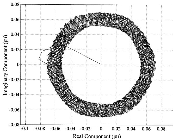
Fig. 13. Space vector of the power transformer's secondary side currents.
