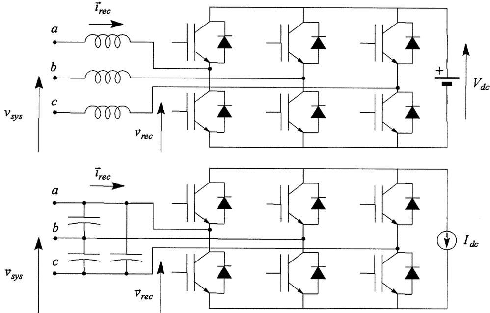
Fig. 7. Active rectifier with a voltage or current source on the dc side.
