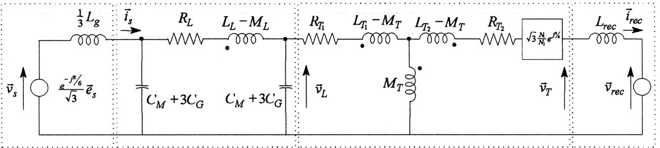
Fig. 10. Space-vector model of the example power system.
