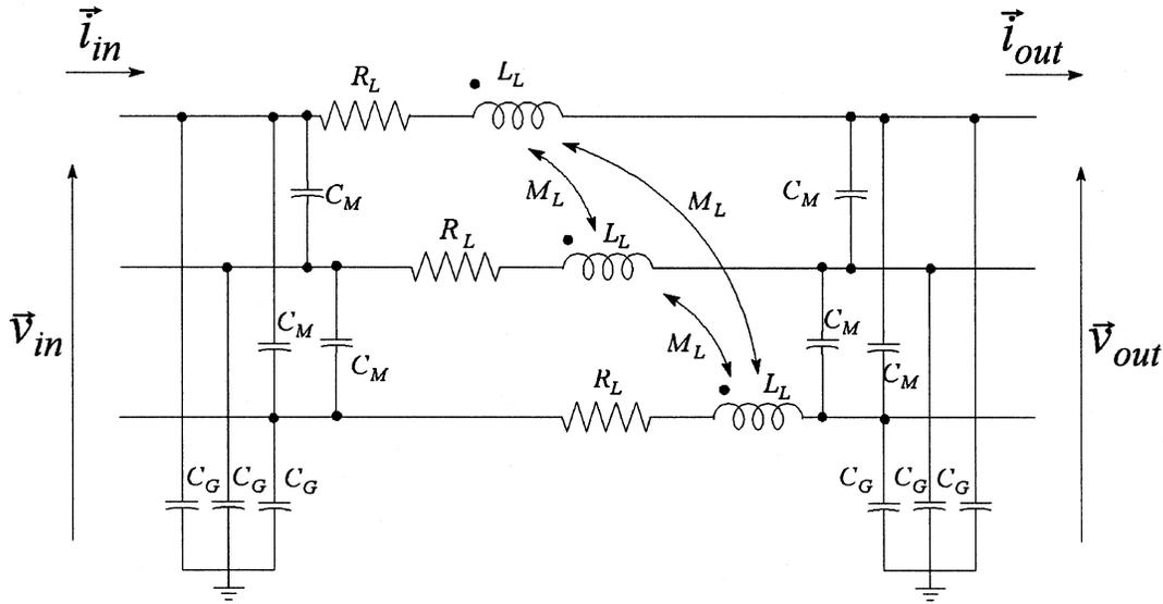
Fig. 3. Medium-length transmission line model.
