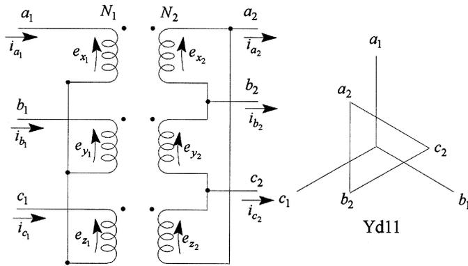
Fig. 4. Ideal three-phase wye-delta transformer.
