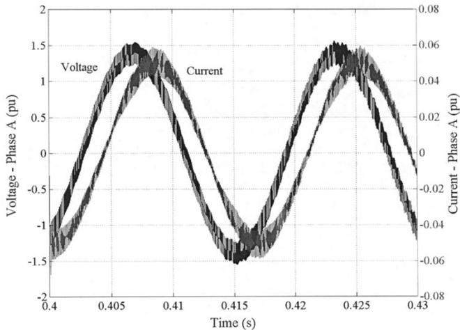
Fig. 15. Instantaneous voltage and current in one phase of the power transformer's secondary side. Power system simulation example, with transients and harmonics included.
