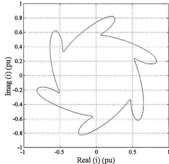
Fig. 17. Space vector of the load current in steady state.
