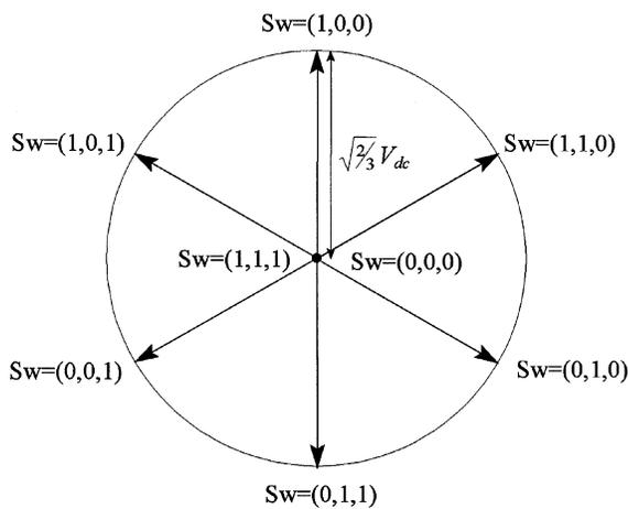
Fig. 8. Voltage spatial vector  $\vec{v}_{sec}$  as function of the switching vector  $\mathbf{Sw}$  for a rectifier bridge feeding a voltage source.
