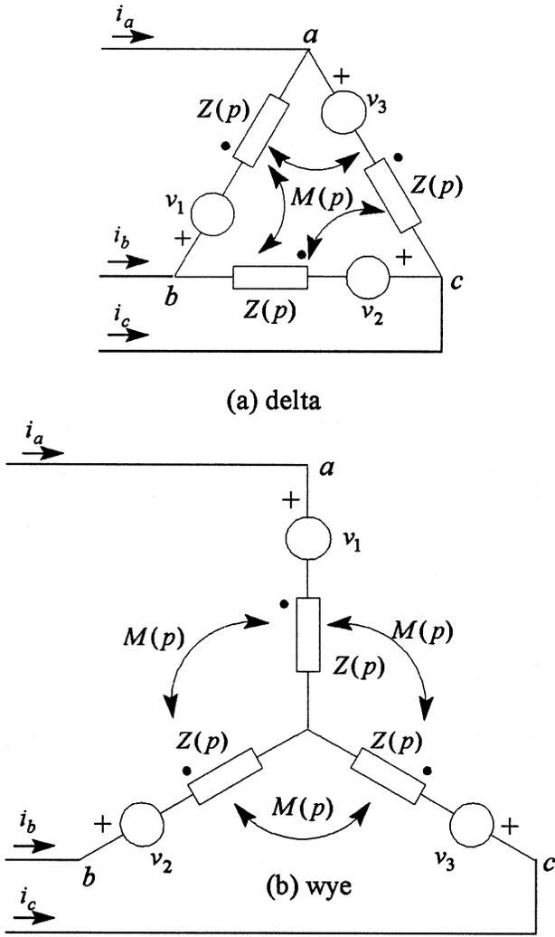
Fig. 2. Operational loads and simple sources connected in (a) Delta, and (b) Wye.
