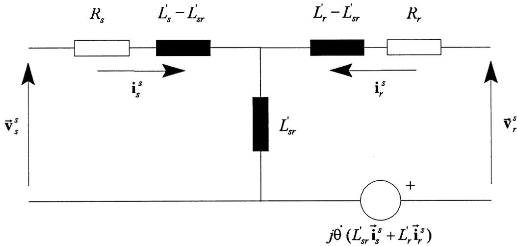
Fig. 6. Space-vector model of the induction machine.
