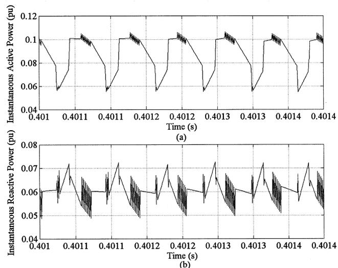
Fig. 14. (a) Instantaneous active power at the transformer's secondary. (b) Instantaneous reactive power at the transformer's secondary.
