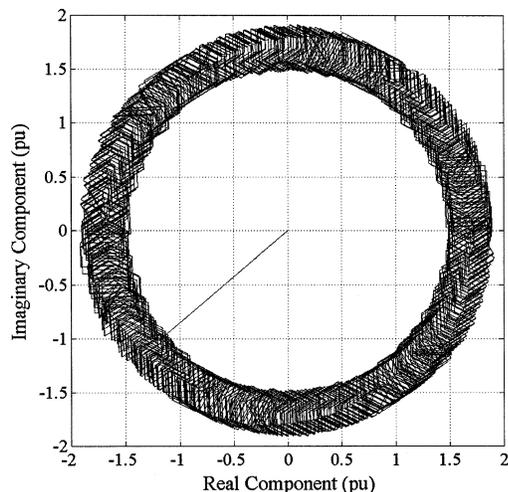
Fig. 12. Space vector of the power transformer's secondary side voltage.
