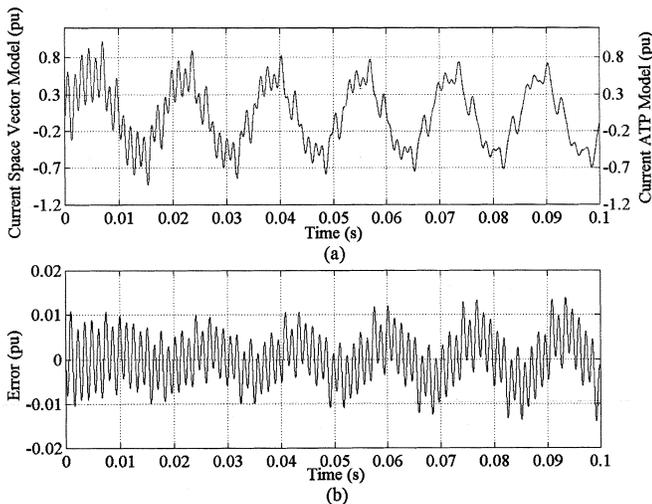
Fig. 16. (a) Instantaneous current in phase "a" of the load. ATP and space-vector models. (b) Instantaneous error between ATP and space-vector models.
