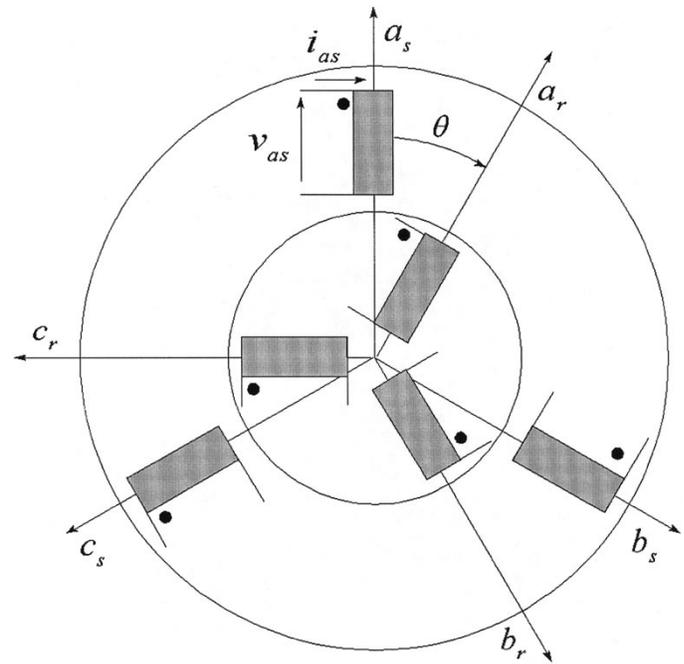
Fig. 5. Three-phase induction machine.
