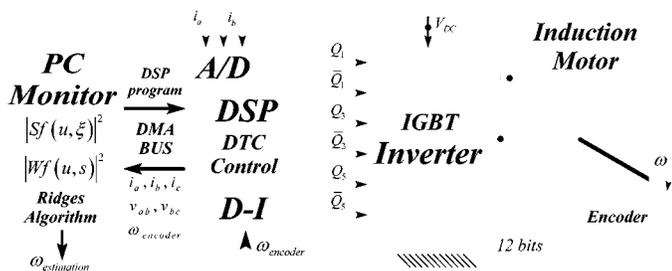
Fig. 3. Block diagram of the experimental system.
