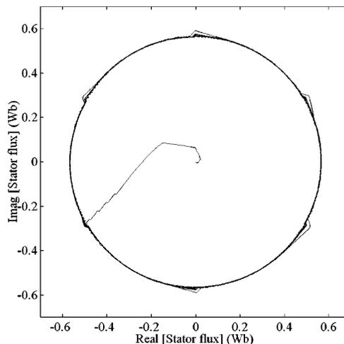
Fig. 6. Space vector of the stator flux during startup with a DTC drive (constant torque and flux references).
