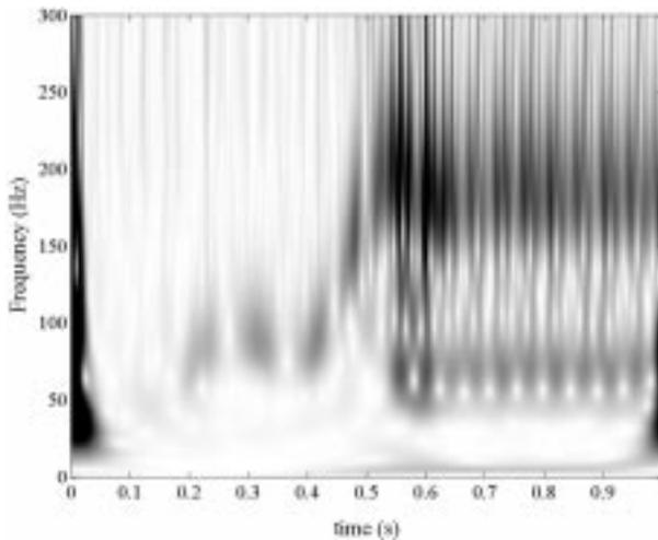
Fig. 13. AWT spectrogram of the stator current.
