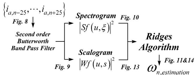
Fig. 4. Speed observer algorithm.
