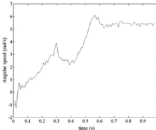
Fig. 7. Angular speed of the induction machine during startup measured with an optical encoder.
