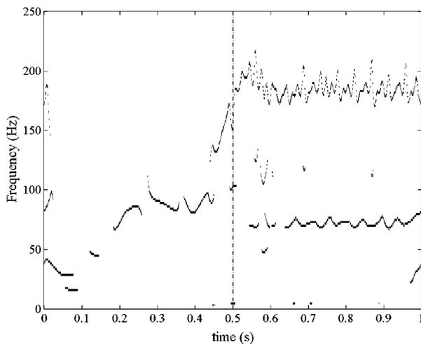
Fig. 14. Ridges of the AWT spectrogram of the stator current.
