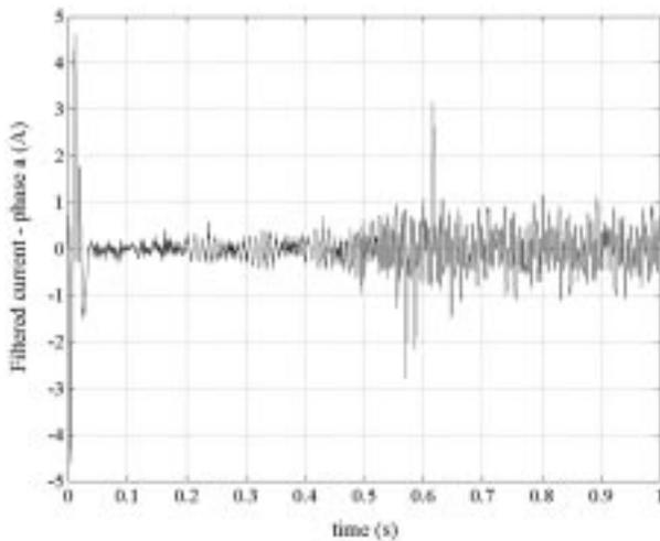
Fig. 9. Stator current processed by the second-order Butterworth bandpass filter.
