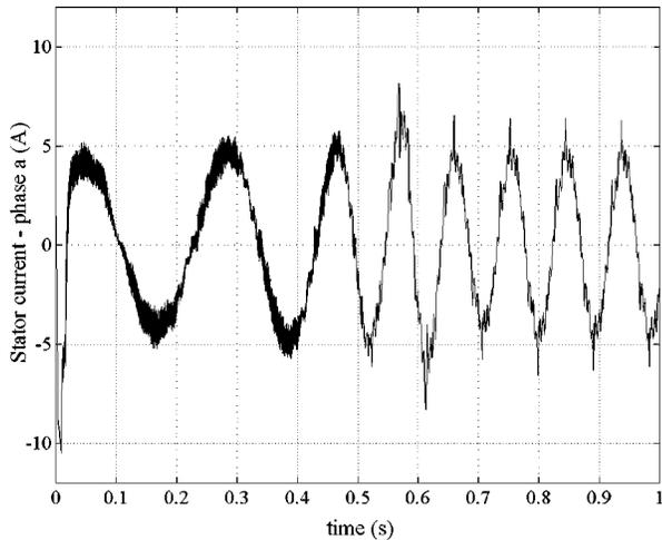
Fig. 8. Stator current of the induction machine during a DTC startup with constant torque and flux references.
