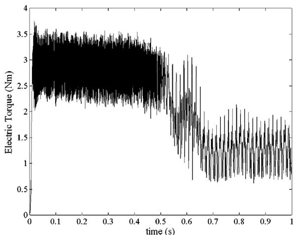
Fig. 5. Instantaneous electromagnetic torque during startup with a DTC drive (constant torque and flux references).
