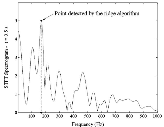
Fig. 12. STFT spectrogram at the instant  $t = 0.5$  s.
