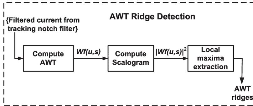
Fig. 2. AWT-ridge-detection algorithm.
