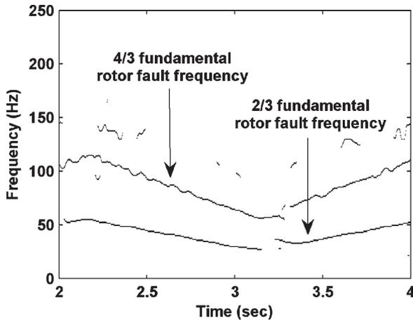
Fig. 12. AWT scalogram of filtered BLDC motor (with dynamic eccentricity) stator current with 5-Hz triangular speed reference ( $\eta = 6$  and  $\sigma = 2$ ) depicting better frequency discrimination than Fig. 11.
