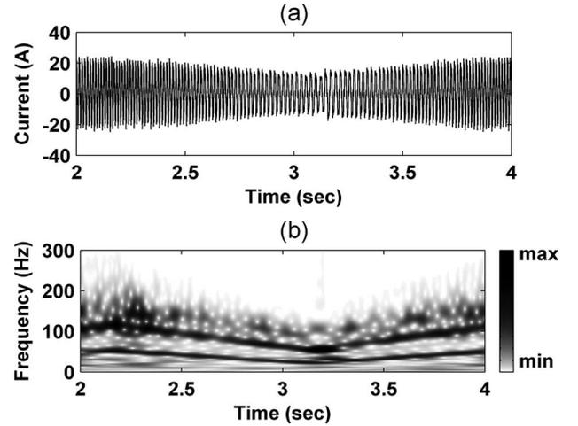
Fig. 6. AWT scalogram of filtered BLDC motor (with dynamic eccentricity) stator current with 5-Hz triangular speed reference.
