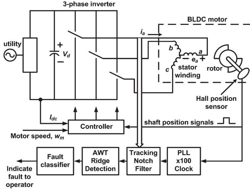
Fig. 1. AWT-ridge-based BLDC rotor-fault detector.
