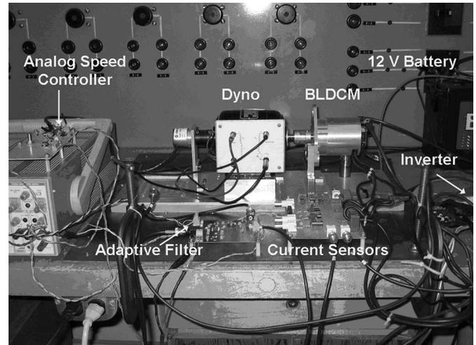
Fig. 4. Experimental arrangement for testing dynamic eccentricity.
