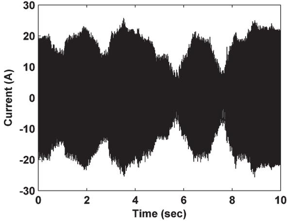
Fig. 5. Nonstationary stator current of a BLDC motor (with dynamic eccentricity).
