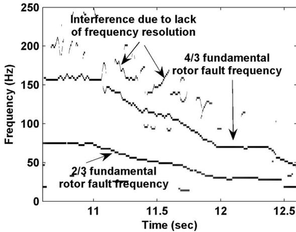
Fig. 9. AWT ridges of filtered stator current in BLDC motor operating with continuous random speed reference.
