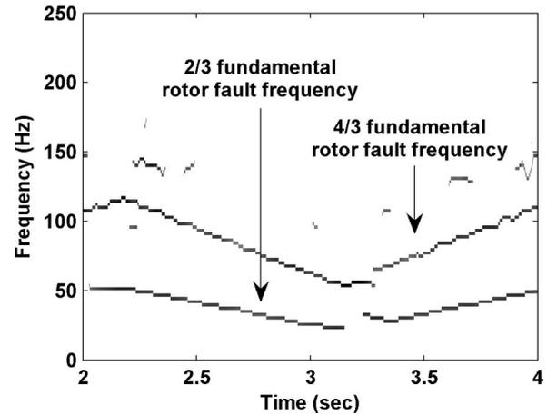
Fig. 7. AWT-ridge extraction from filtered stator current scalogram in BLDC motor operating with 5-Hz triangular speed reference.
