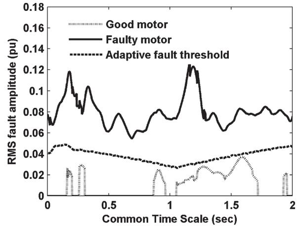
Fig. 10. AWT-ridge-based BLDC rotor-fault detector using rms fault metric.
