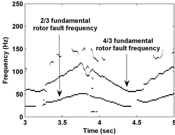
Fig. 8. AWT ridges of filtered stator current in BLDC motor operating with 8-Hz triangular speed reference.
