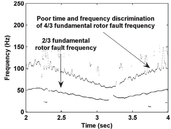
Fig. 11. AWT scalogram of filtered BLDC motor (with dynamic eccentricity) stator current with 5-Hz triangular speed reference ( $\eta = 6$  and  $\sigma = 1$ ) depicting poor frequency discrimination.
