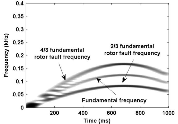
Fig. 2. WFT of simulated BLDCM rotor fault using hypothetical test signal  $i_a$ .
