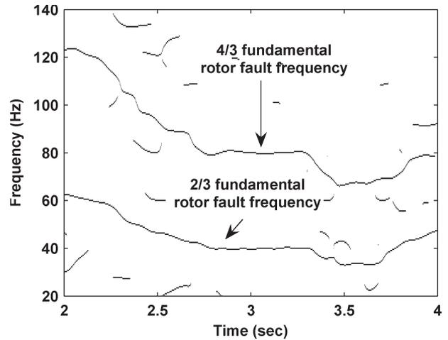
Fig. 19. Windowed Fourier ridges of filtered BLDCM (with dynamic eccentricity) stator current and random speed reference.
