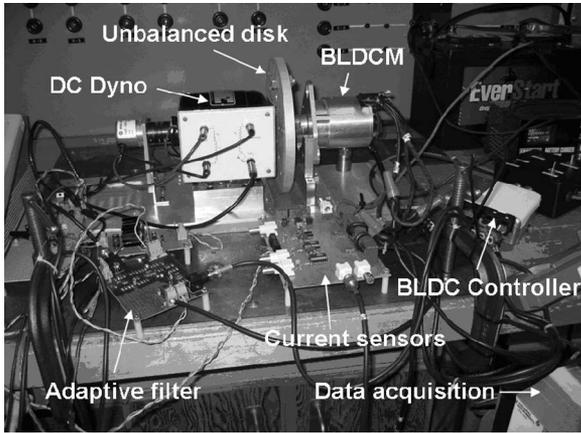
Fig. 7. Experimental arrangement to test fault detection in dynamically operating BLDCMs.
