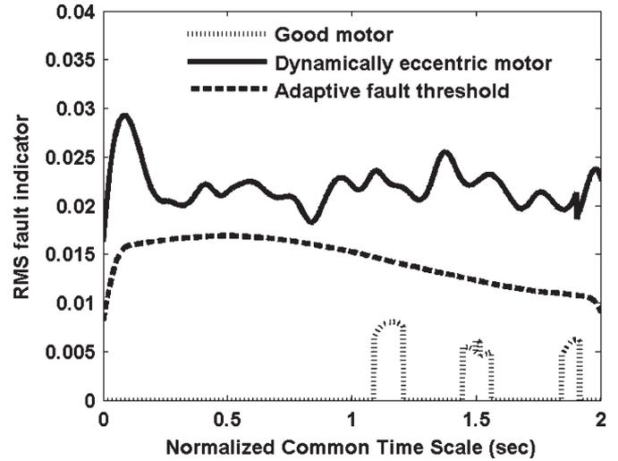
Fig. 23. Detecting dynamic eccentricity with adaptive threshold set at 2% of the fundamental amplitude (3-Hz sine speed reference) for time segment different from Fig. 22.
