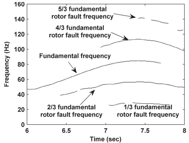
Fig. 11. Windowed Fourier ridges of filtered BLDCM (with a mechanically unbalanced rotor) stator current and 3-Hz sine speed reference.
