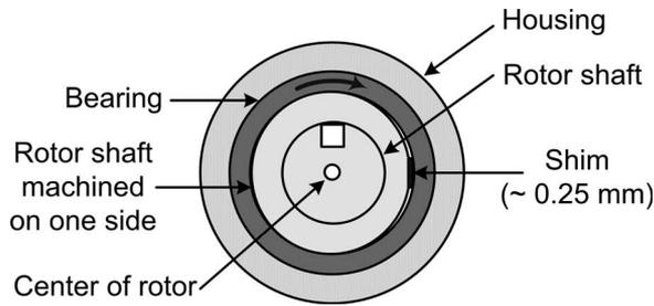
Fig. 13. Laboratory implementation of dynamic eccentricity
