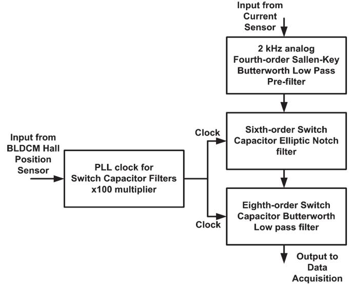
Fig. 9. Block diagram of ATF.
