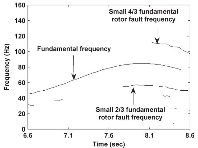
Fig. 12. Windowed Fourier ridges of filtered BLDCM (with mechanically balanced rotor) stator current and 3-Hz sine speed reference.
