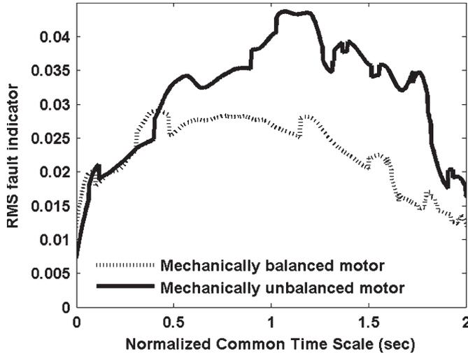
Fig. 21. RMS fault indicator discriminates BLDC rotor unbalance (3-Hz sine speed reference).
