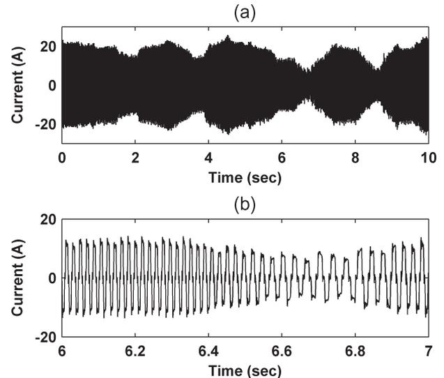
Fig. 1. (a) Nonstationary stator current in BLDCM. (b) Zoomed section of top plot depicting continuously changing motor frequency and amplitude.
