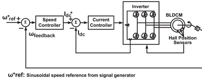
Fig. 8. Detailed block diagram of BLDCM controller.
