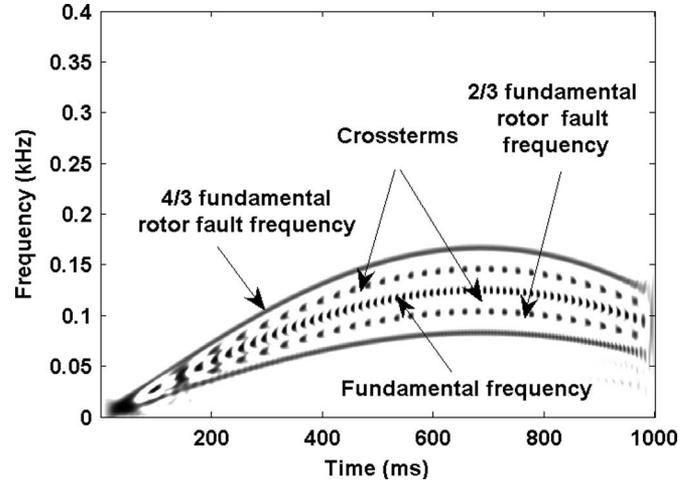
Fig. 3. PWVD of simulated BLDCM rotor fault using hypothetical test signal  $i_a$ .
