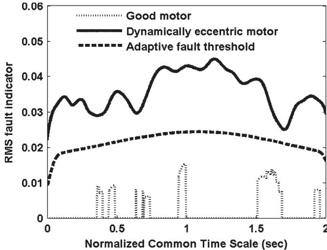
Fig. 22. Detecting dynamic eccentricity with adaptive threshold set at 2% of the fundamental amplitude (3-Hz sine speed reference).
