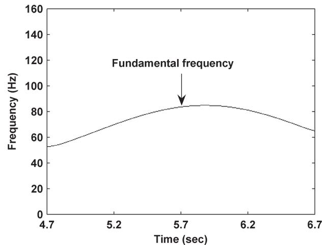
Fig. 15. Windowed Fourier ridges of unfiltered BLDCM (with dynamic eccentricity) stator current and 3-Hz sine speed reference.
