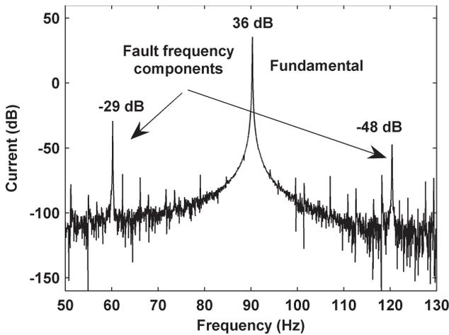
Fig. 6. Attenuation of fault sidebands with respect to fundamental for case of BLDCM with dynamic eccentricity.
