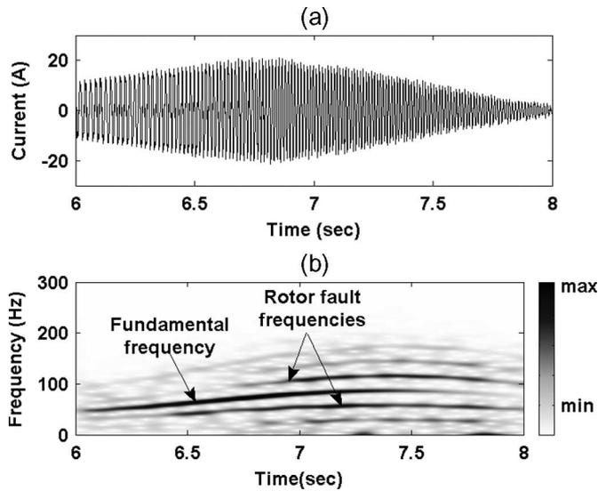
Fig. 10. Nonstationary BLDCM stator current and spectrogram of corresponding filtered BLDCM (with mechanically unbalanced rotor) stator current with 3-Hz sine speed reference.
