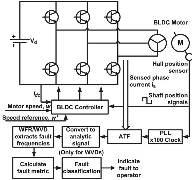
Fig. 5. Rotor fault detection in BLDCMs operating under nonstationary conditions.
