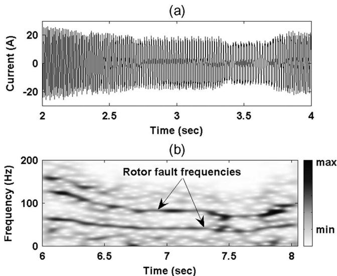
Fig. 18. Nonstationary BLDCM stator current and spectrogram of corresponding filtered BLDCM (with dynamic eccentricity) stator current with random speed reference.
