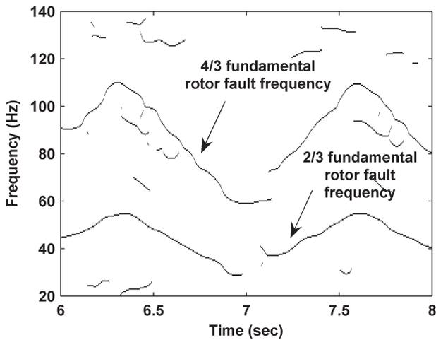
Fig. 17. Windowed Fourier ridges of filtered BLDCM (with dynamic eccentricity) stator current and 8-Hz triangular speed reference.
