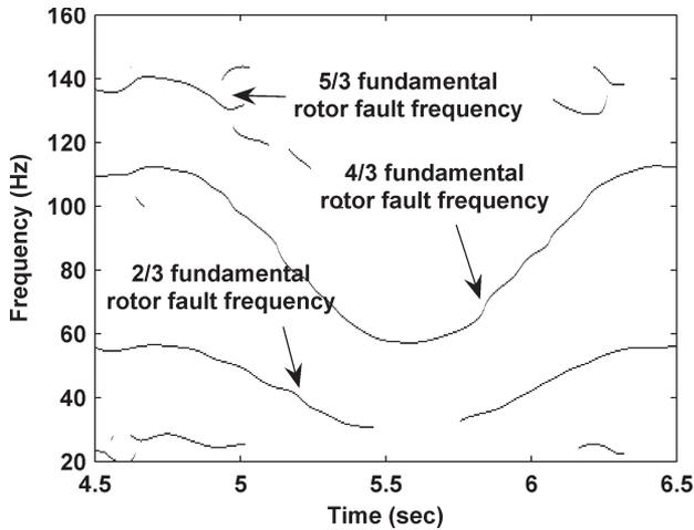
Fig. 16. Windowed Fourier ridges of filtered BLDCM (with dynamic eccentricity) stator current and 6-Hz sine speed reference.
