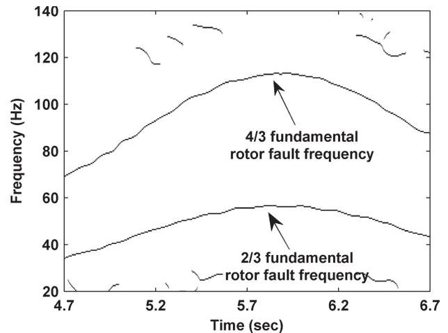
Fig. 14. Windowed Fourier ridges of filtered BLDCM (with dynamic eccentricity) stator current and 3-Hz sine speed reference.
