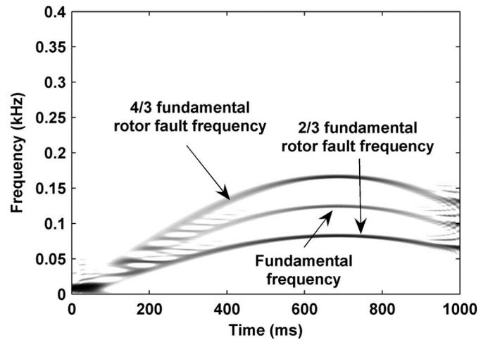
Fig. 4. SPWVD of simulated BLDCM rotor fault using hypothetical test signal  $i_a$ .
