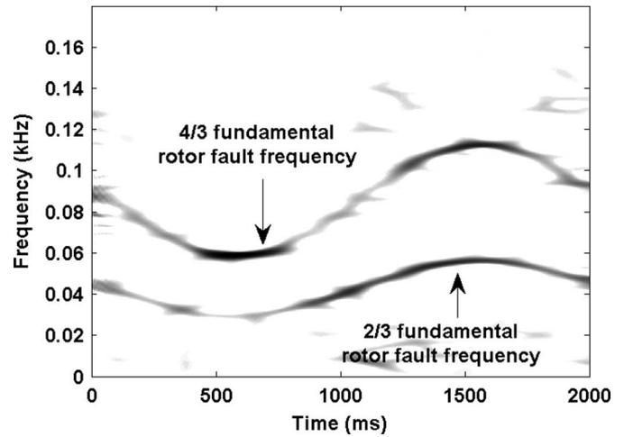
Fig. 20. SPWVD of BLDCM with dynamic eccentricity (5-Hz sinusoidal speed reference).
