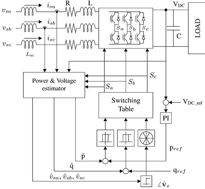
Fig. 1. Block diagram of the classical DPC.
