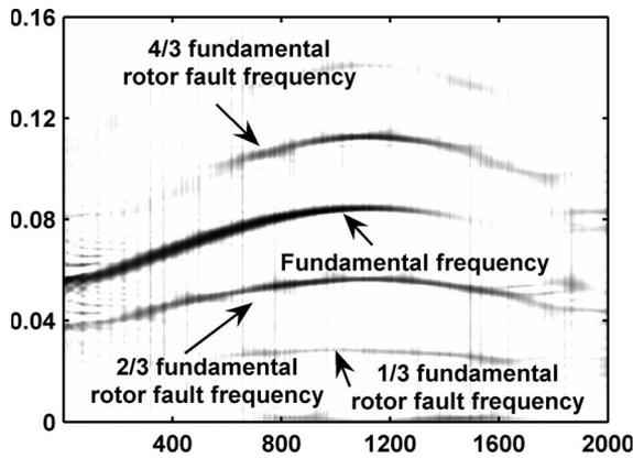
Fig. 8. CWD of filtered BLDCM (with mechanical unbalanced rotor) stator current and 3-Hz sine speed reference.
