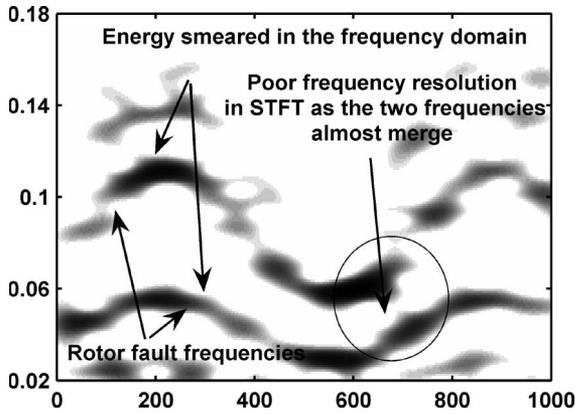
Fig. 13. STFT of filtered BLDCM (with dynamic eccentricity) stator current and 15-Hz sinusoidal speed reference.
