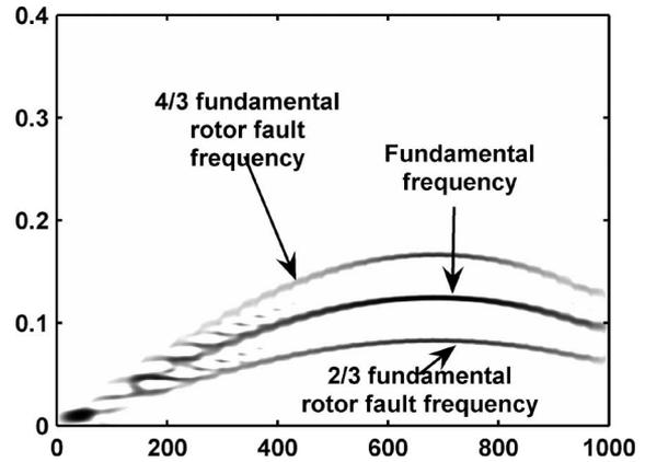
Fig. 7. ZAM of simulated BLDCM rotor fault comprising of three frequencies varying over time.
