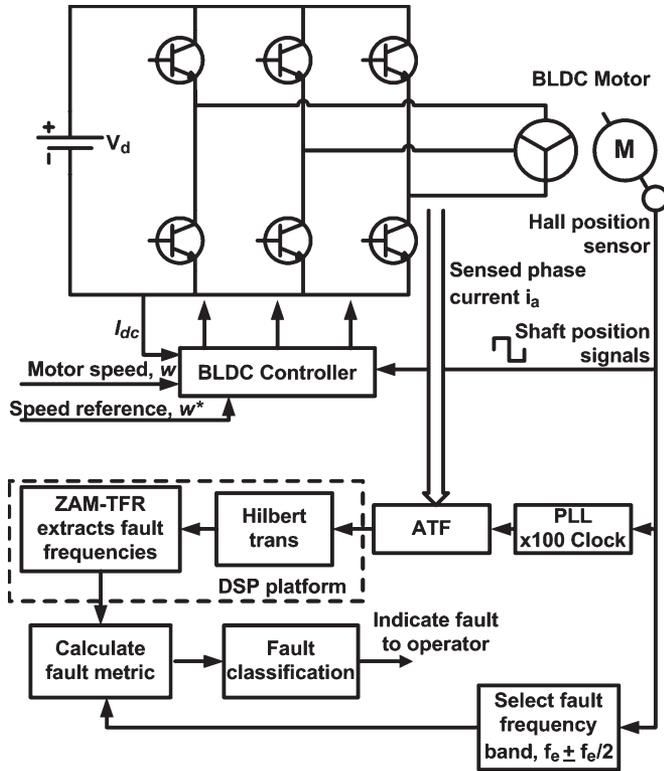
Fig. 2. Fault detection in BLDCMs using TFRs.
