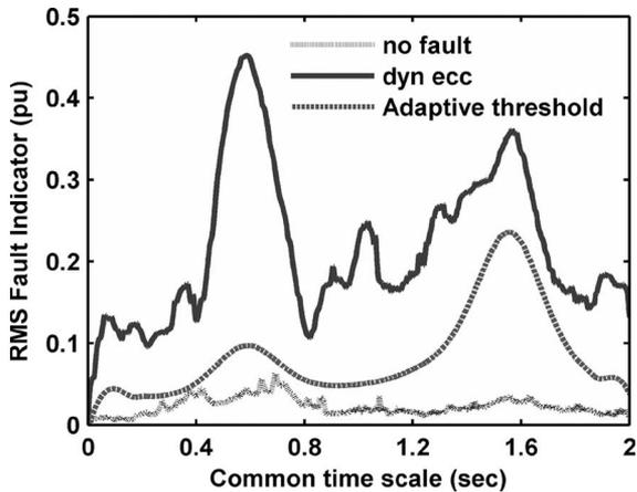
Fig. 14. RMS fault indicator discriminates the BLDC rotor eccentricity using an adaptive threshold (5-Hz sinusoidal speed reference).
