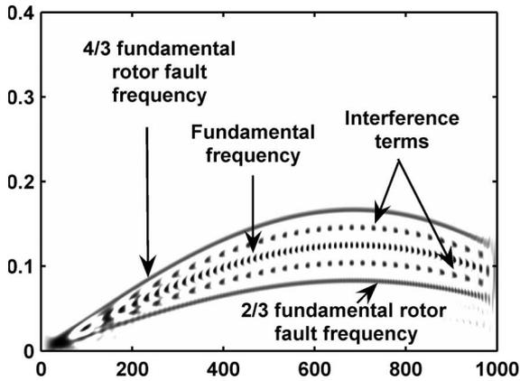
Fig. 4. PWVD of simulated BLDCM rotor fault comprising of three frequencies varying over time.
