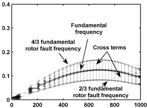
Fig. 6. BJD of simulated BLDCM rotor fault comprising of three frequencies varying over time.
