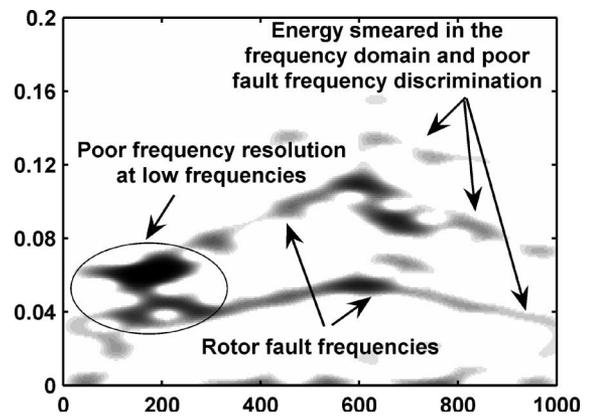
Fig. 11. STFT of filtered BLDCM (with dynamic eccentricity) stator current and 10-Hz triangular speed reference.
