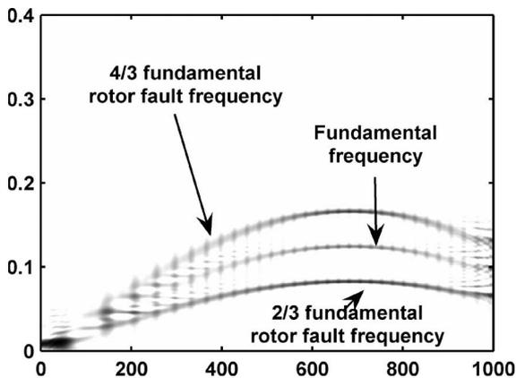
Fig. 5. CWD of simulated BLDCM rotor fault comprising of three frequencies varying over time.
