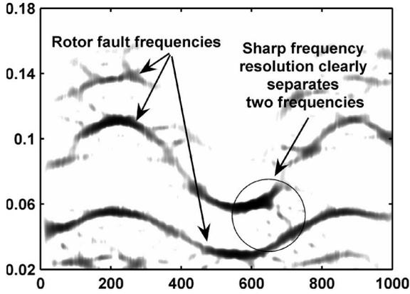
Fig. 12. ZAM of filtered BLDCM (with dynamic eccentricity) stator current and 15-Hz sinusoidal speed reference.
