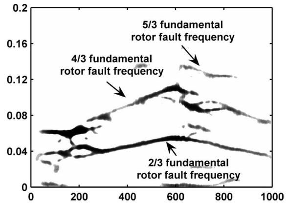
Fig. 10. ZAM of filtered BLDCM (with dynamic eccentricity) stator current and 10-Hz triangular speed reference.
