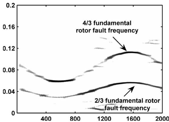
Fig. 9. ZAM of filtered BLDCM (with dynamic eccentricity) stator current and 5-Hz sinusoidal speed reference.
