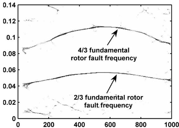
Fig. 15. Reassigned SPWV of filtered BLDCM (with dynamic eccentricity) stator current and 5-Hz sinusoidal speed reference.
