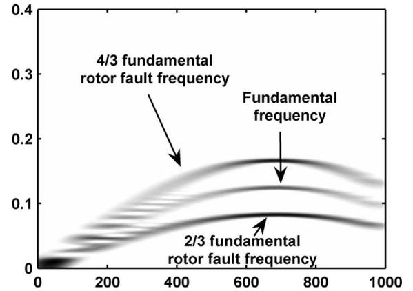
Fig. 3. STFT of simulated BLDCM rotor fault comprising of three frequencies varying over time.
