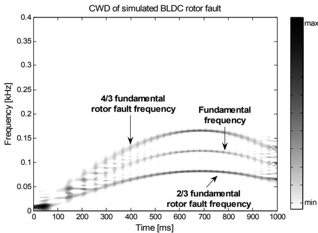
Fig. 3. CWD of simulated BLDCM rotor fault.
