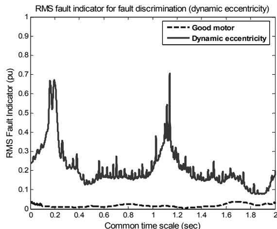
Fig. 9. RMS fault indicator discriminates BLDC rotor eccentricity (5 Hz triangular speed ref).
