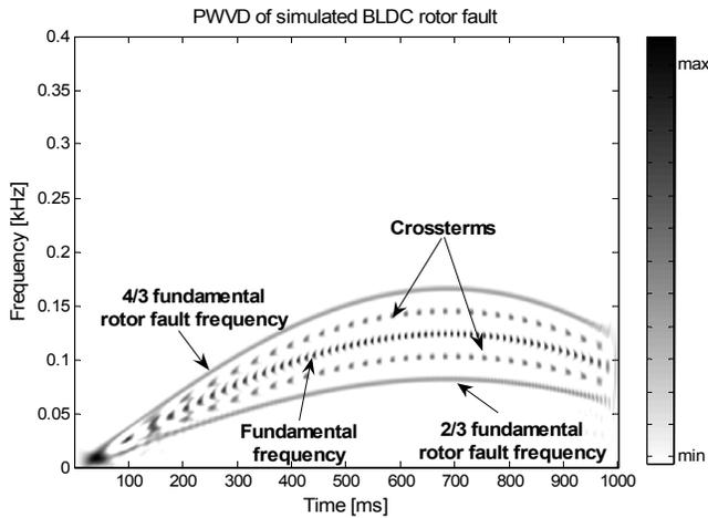
Fig. 2. PWVD of simulated BLDCM rotor fault.
