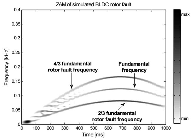
Fig. 4. ZAM of simulated BLDCM rotor fault.
