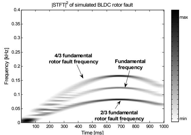
Fig. 1. STFT of simulated BLDCM rotor fault.
