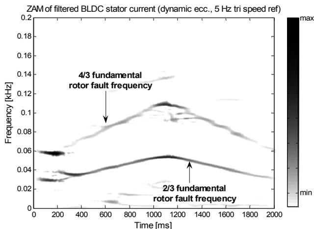
Fig. 8. ZAM of filtered BLDC motor (with dynamic eccentricity) stator current and 5 Hz triangular speed reference..
