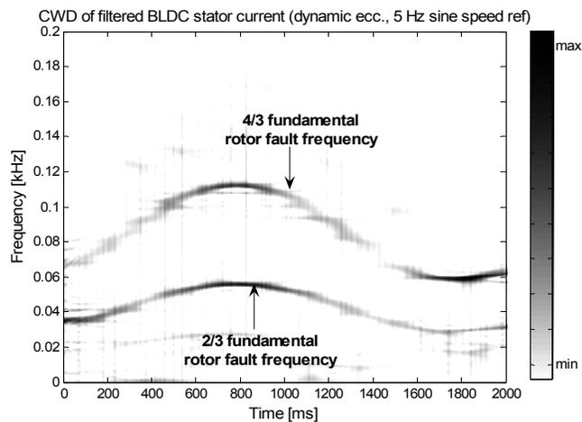
Fig. 7. CWD of filtered BLDC motor (with dynamic eccentricity) stator current and 5 Hz sine speed reference.
