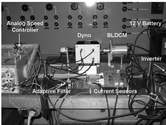
Fig. 5. Experimental arrangement for testing dynamic eccentricity.
