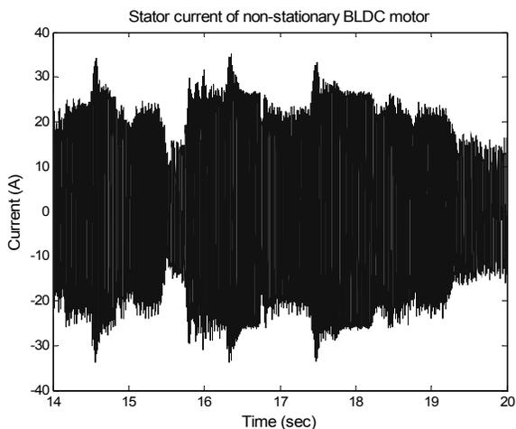
Fig. 6. Non-stationary stator current in a BLDC motor.
