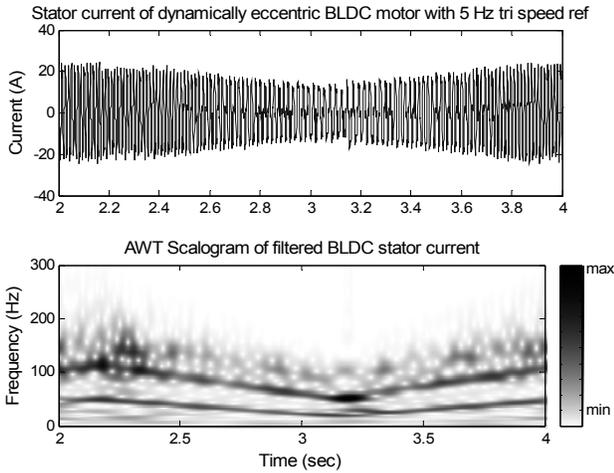
Fig. 6. AWT scalogram of filtered BLDC motor (with dynamic eccentricity) stator current with 5 Hz triangular speed reference.
