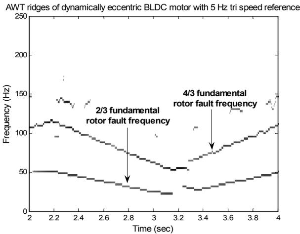
Fig. 7. AWT ridge extraction from filtered stator current scalogram in BLDC motor operating with 5 Hz triangular speed reference.
