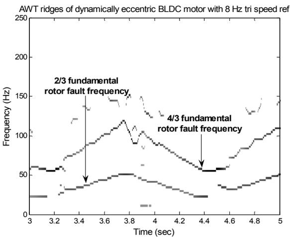
Fig. 8. AWT ridges of filtered stator current in BLDC motor operating with 8 Hz triangular speed reference.
