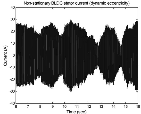
Fig. 5. Non-stationary stator current of a BLDC motor (with dynamic eccentricity).
