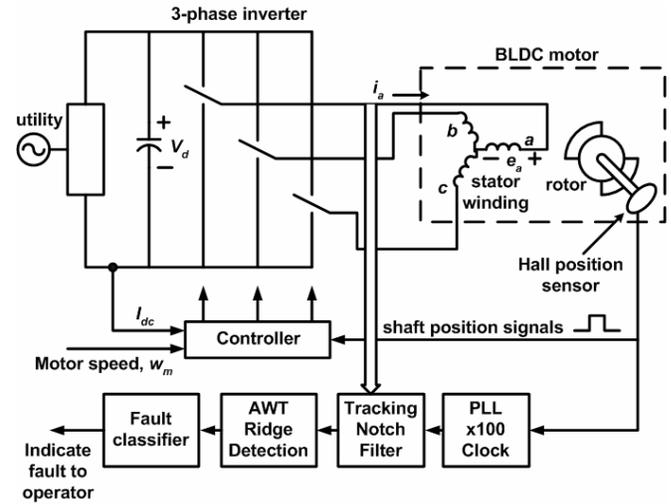
Fig. 1. AWT ridge based BLDC rotor fault detector.
