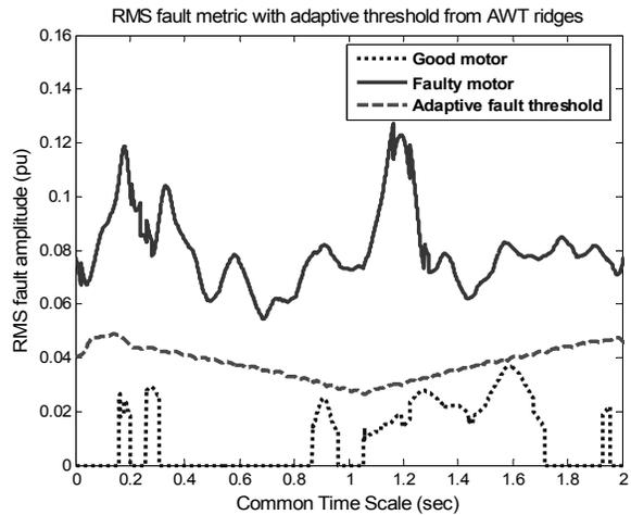
Fig. 10. AWT ridge based BLDC rotor fault detector using RMS fault metric.
