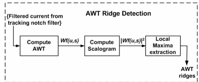
Fig. 2. AWT ridge detection algorithm.
