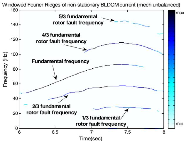
Figure 7. Windowed Fourier ridges of filtered BLDC motor (with mech. unbalanced rotor) stator current and 3 Hz sine speed reference.
