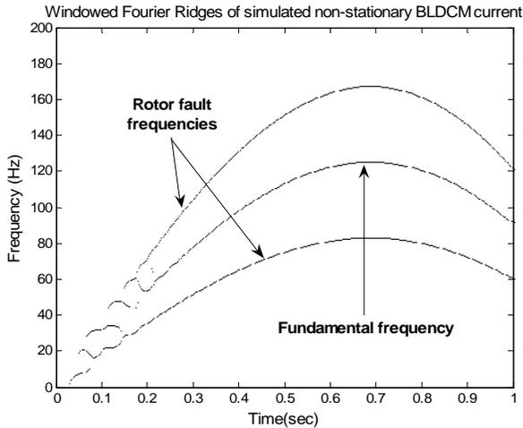
Figure 2. Windowed Fourier ridges of simulated non-stationary stator current in a faulty BLDC motor.
