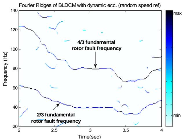
Figure 15. Windowed Fourier ridges of filtered BLDC motor (with dynamic eccentricity) stator current and random speed reference.
