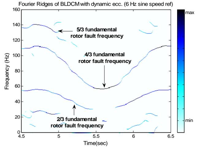
Figure 12. Windowed Fourier ridges of filtered BLDC motor (with dynamic eccentricity) stator current and 6 Hz sine speed reference.
