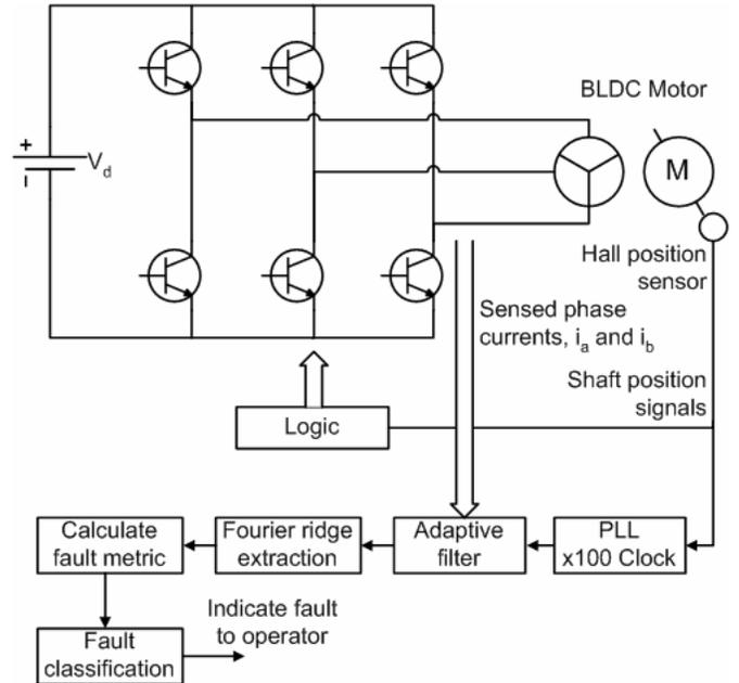
Figure 3. Rotor fault detection in BLDC motors using windowed Fourier ridge algorithm.
