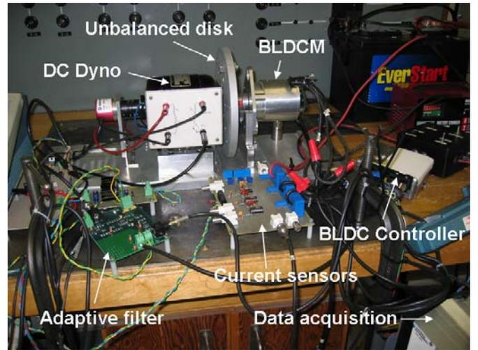
Figure 4. Experimental arrangement to test fault detection in dynamically operating BLDC motors.
