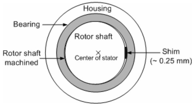
Figure 10. Laboratory implementation of dynamic eccentricity.
