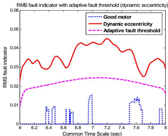
Figure 16. Detecting dynamic eccentricity with adaptive threshold set at 2% of fundamental amplitude (3 Hz sine speed reference).
