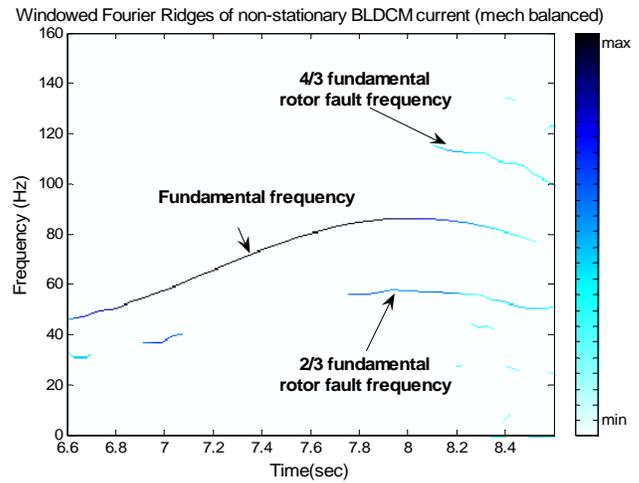
Figure 8. Windowed Fourier ridges of filtered BLDC motor (with mech. balanced rotor) stator current and 3 Hz sine speed reference.
