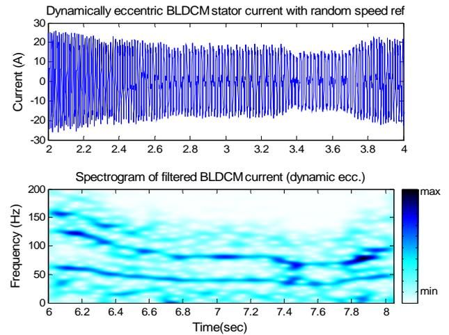
Figure 14. Non-stationary BLDC motor stator current and the spectrogram of the corresponding filtered BLDC motor (with dynamic eccentricity) stator current with random speed reference.
