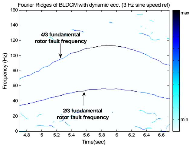
Figure 11. Windowed Fourier ridges of filtered BLDC motor (with dynamic eccentricity) stator current and 3 Hz sine speed reference.
