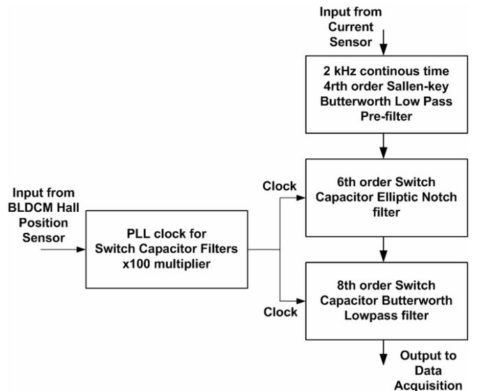
Figure 5. Block diagram of analog tracking filter.
