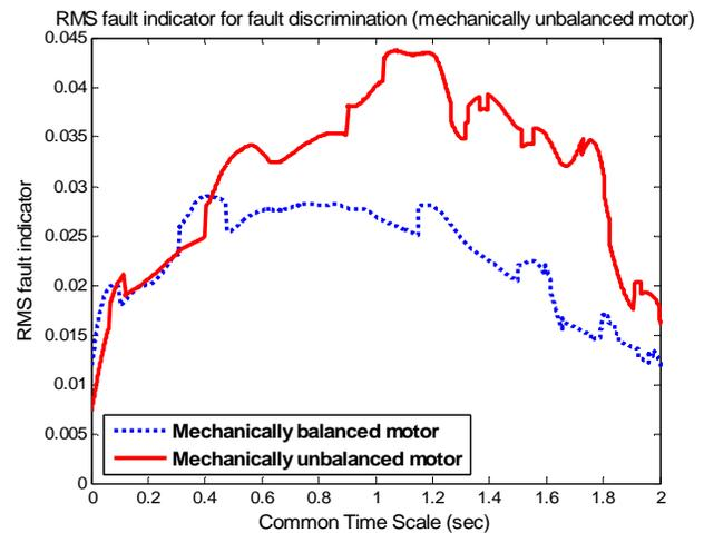
Figure 9. RMS fault indicator discriminates BLDC rotor unbalance (3 Hz sine speed ref).
