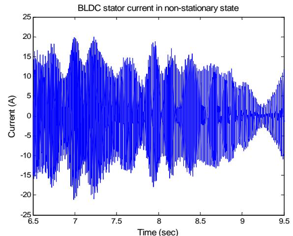
Figure 1. Non-stationary stator current in a BLDC motor.
