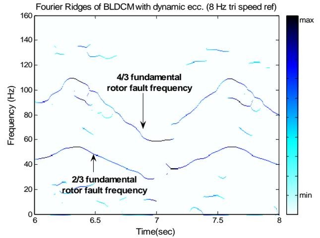
Figure 13. Windowed Fourier ridges of filtered BLDC motor (with dynamic eccentricity) stator current and 8 Hz triangular speed reference.
