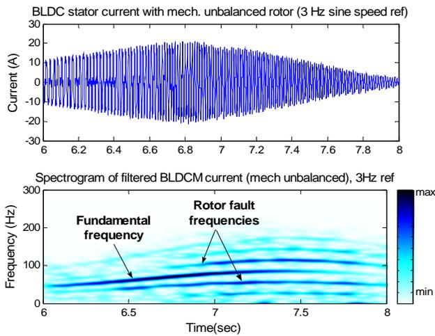
Figure 6. Non-stationary BLDC motor stator current and the spectrogram of the corresponding filtered BLDC motor (with mechanically unbalanced rotor) stator current with 3 Hz sine speed reference.
