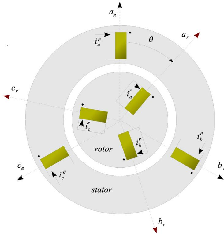
Figure 1: Induction Machine in “abc” coordinates frame
