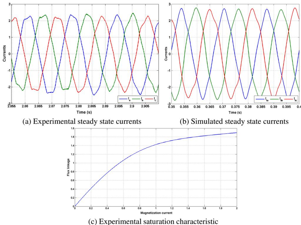
Figure 6: Comparison between experimental and simulated steady state currents using the proposed model
