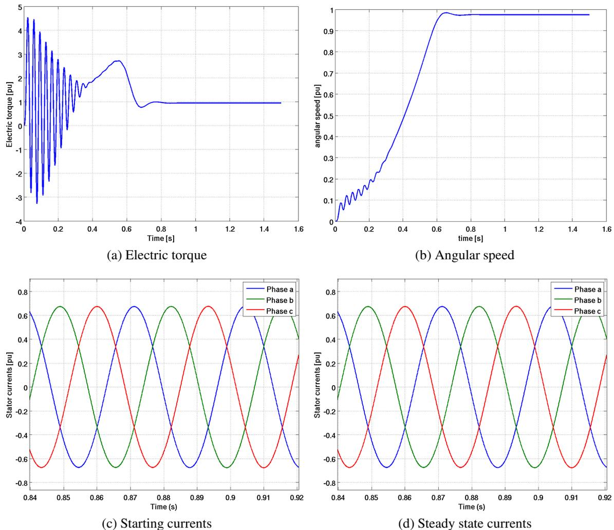
Figure 3: Results obtained with a linear model (no saturation effect)
