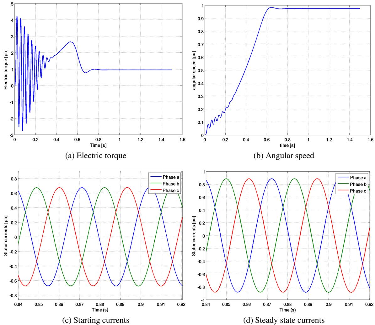
Figure 4: Results obtained with Tang's model (saturated)
