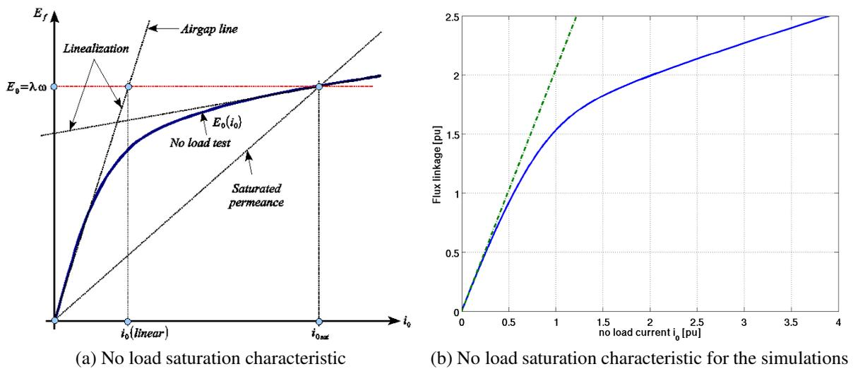
Figure 2: No load saturation test
