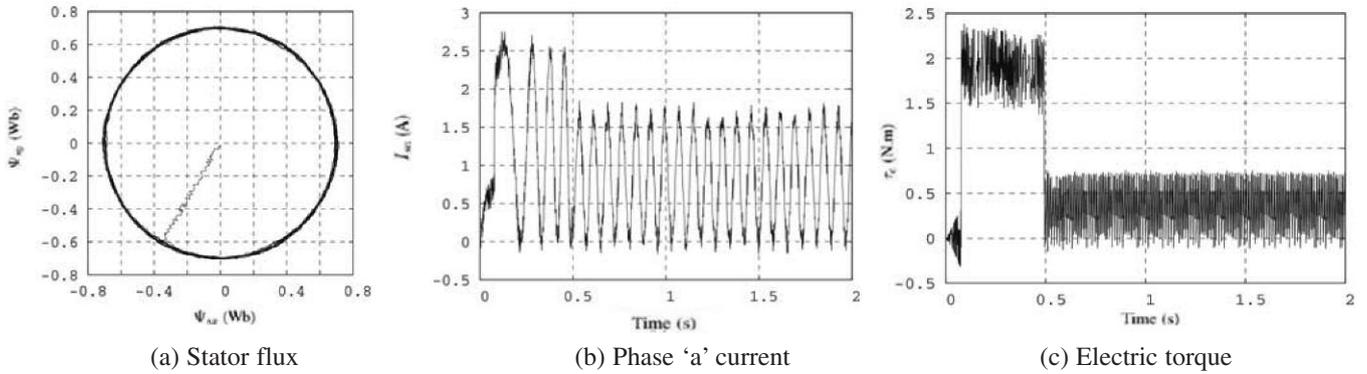
Fig. 9: Simulations for the DTC with medium size space vectors set
