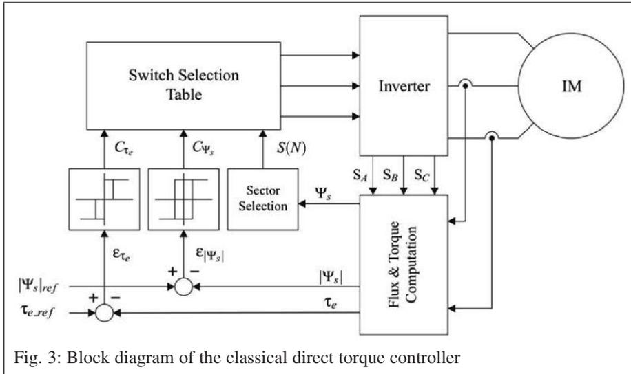
Fig. 3: Block diagram of the classical direct torque controller
