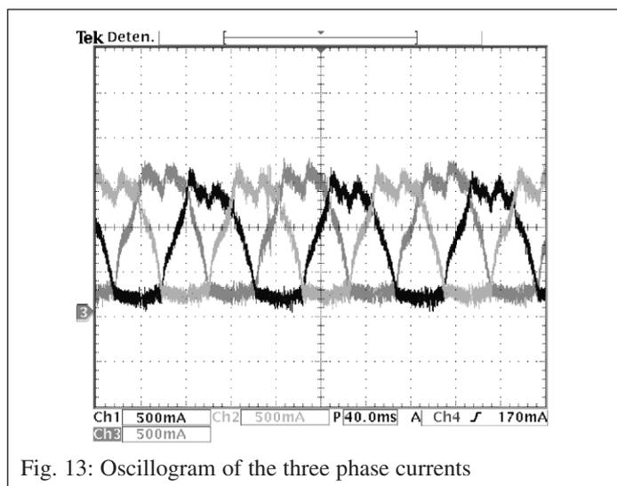
Fig. 13: Oscillogram of the three phase currents
