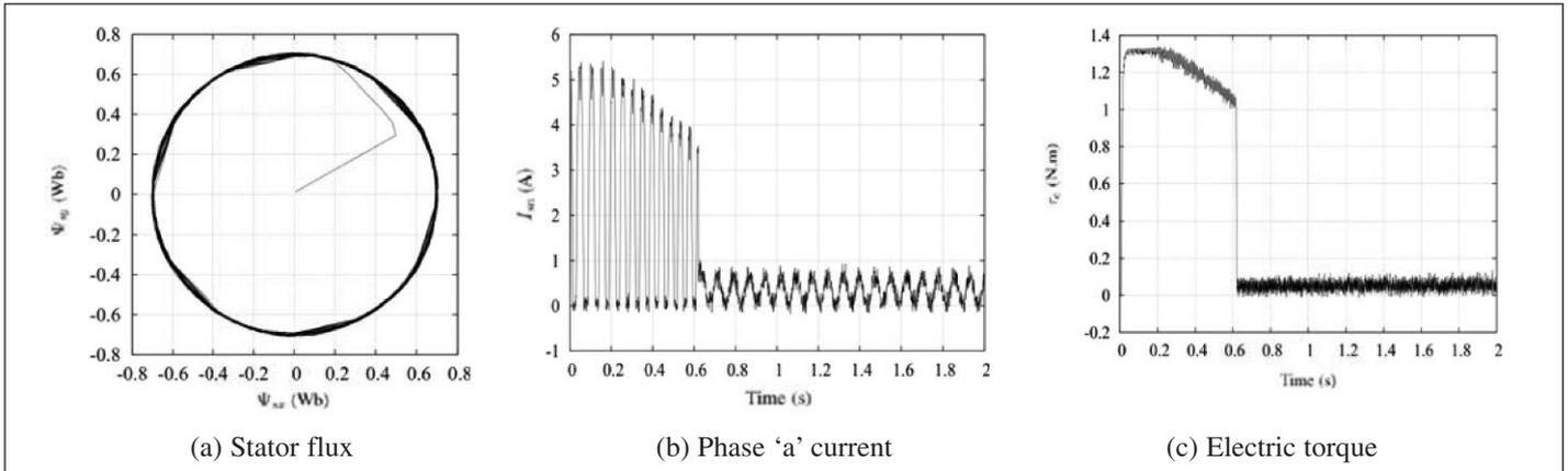
Fig. 11: Simulations for the proposed combination of small positive and recovery space vectors sets
