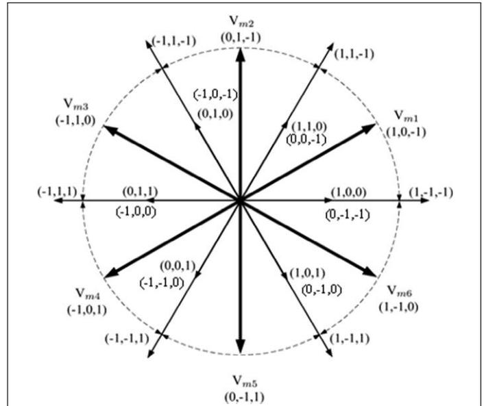
Fig. 2: Space vectors sets for the asymmetric converter
