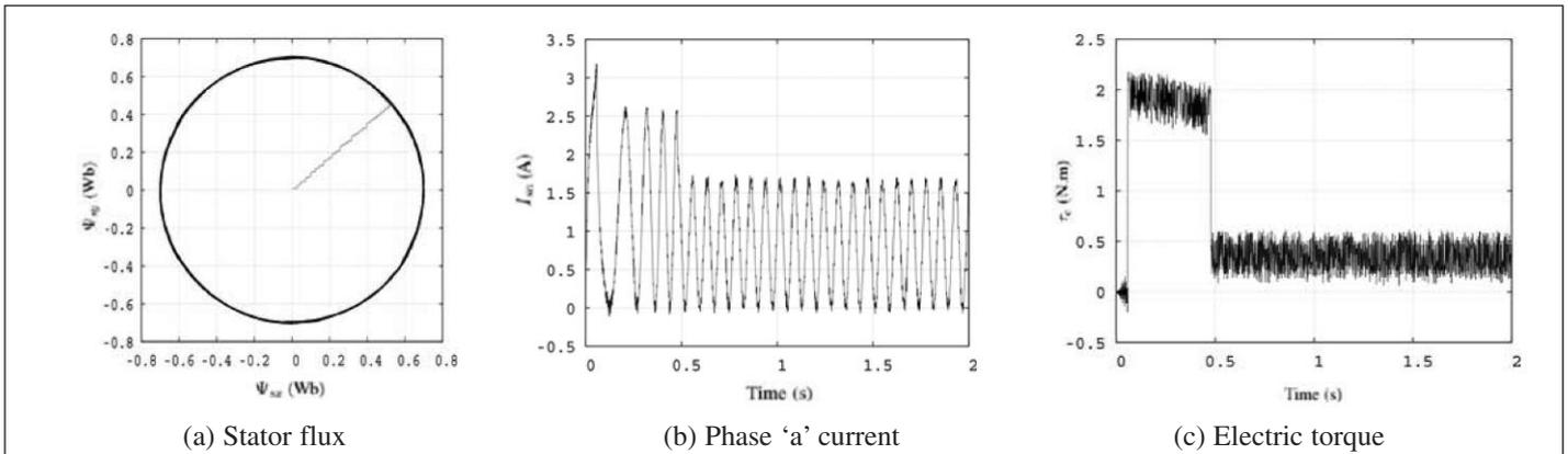
Fig. 5: Simulation results for the DTC with small positive space vectors set
