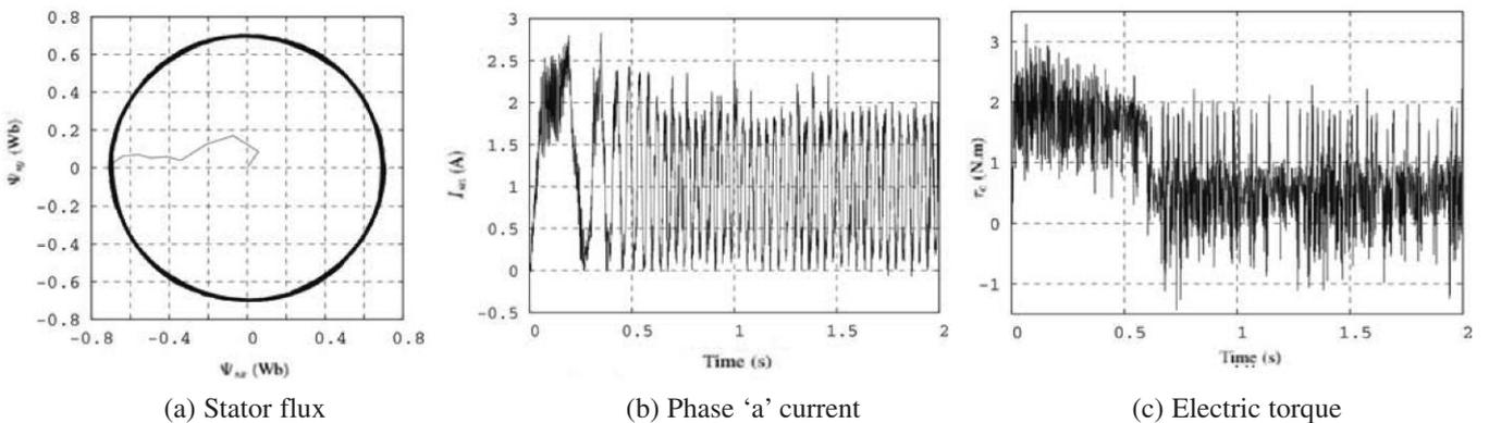
Fig. 10: Experimental results for the DTC with medium size space vectors set
