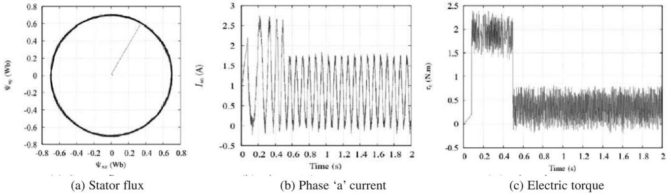
Fig. 7: Simulation results for the DTC with small recovery space vectors set
