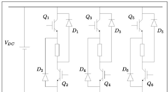
Fig. 1: Circuit diagram of the three phase asymmetric converter
