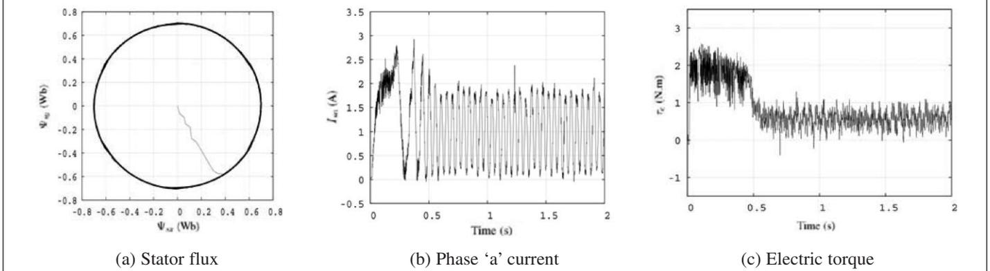
Fig. 6: Experimental results for the DTC with small positive space vectors set
