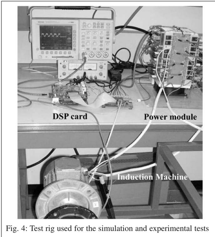
Fig. 4: Test rig used for the simulation and experimental tests
