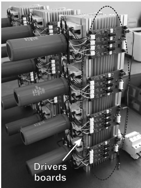
Figure 9: Drivers boards for the IGBTs of converter leg "C".
