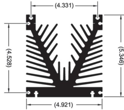
Figure 5: Transverse section of the MM12878 aluminum extrusion profile used as heatsink.
