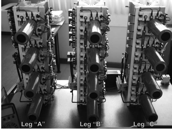
Figure 6: Frontal view of the three converter legs.
