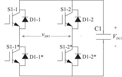
Figure 2: H-bridge block circuit configuration.
