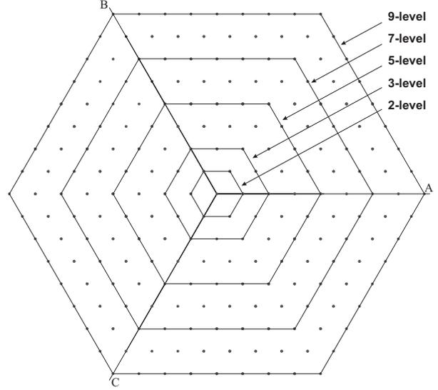
Figure 4: Voltage Space Vectors (VSV) available in converters with different number of voltage levels.
