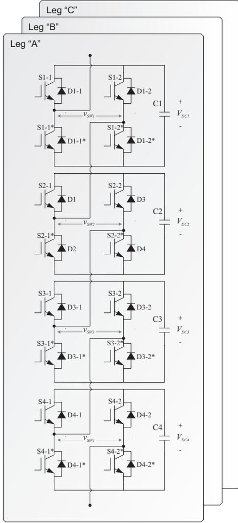
Figure 3: 9-level CHB three legs scheme.
