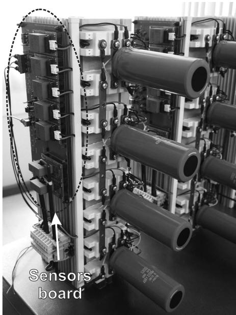
Figure 8: Sensors board attached to converter leg "A".
