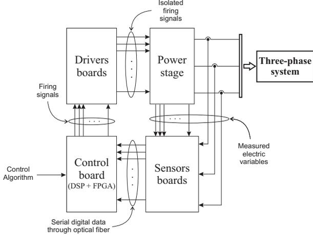
Figure 1: Proposed hardware platform block diagram.
