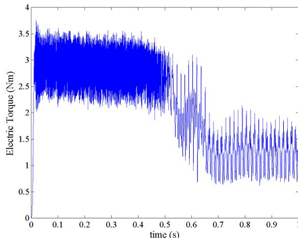
Fig.3. Instantaneous electromagnetic torque during start up with a DTC drive (constant torque and flux references).
