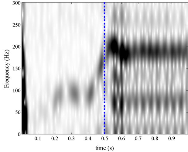
Fig.8. STFT spectrogram of the filtered current obtained using a Gaussian window with 50 points.
