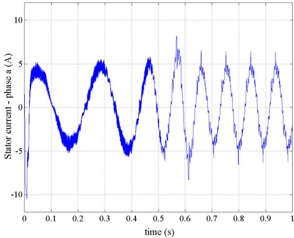
Fig.6. Stator current of the induction machine during a DTC start up with constant torque and flux references.
