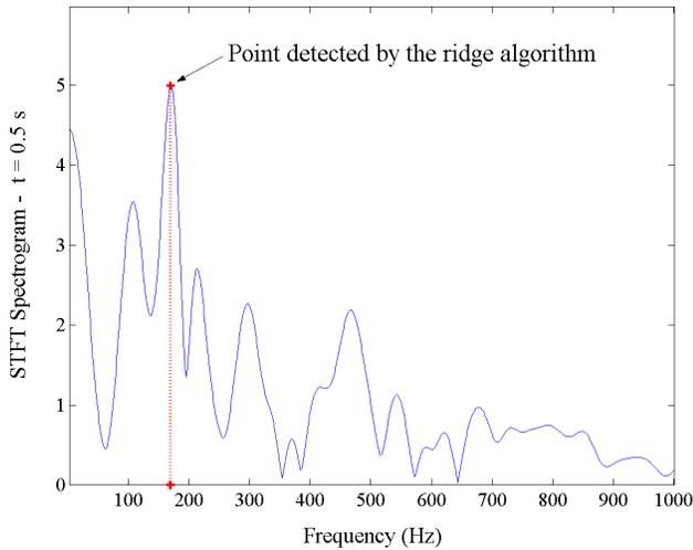
Fig.10. STFT spectrogram at the instant  $t = 0.5$  s.
