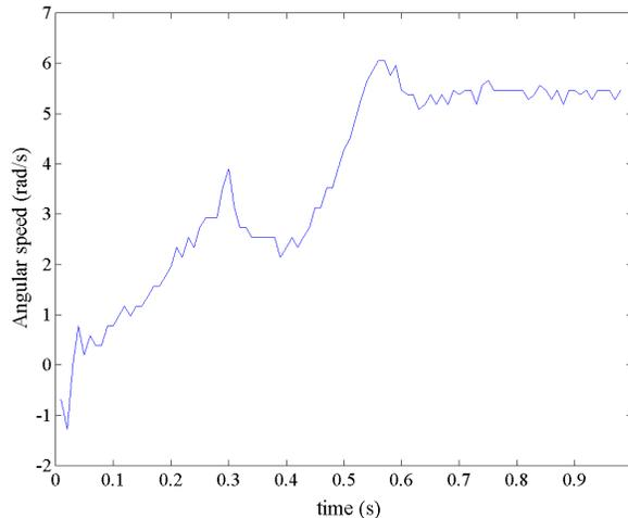
Fig.5. Angular speed of the induction machine during start up measured with an optical encoder.
