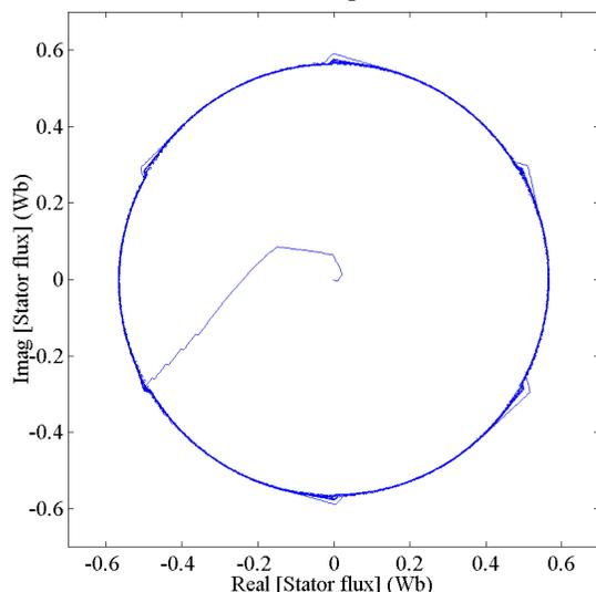
Fig.4. Space vector of the stator flux during start up with a DTC drive (constant torque and flux references).
