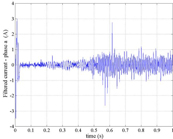
Fig.7. Stator current processed by the second order butterworth band pass filter.
