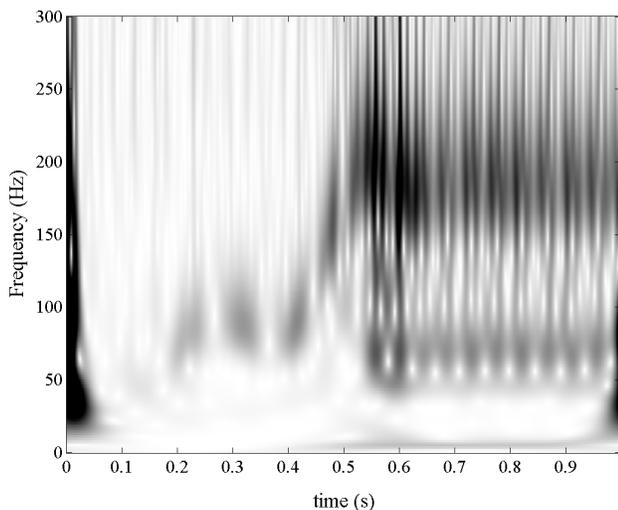
Fig.11. AWT spectrogram of the stator current
