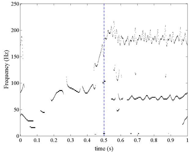
Fig.12. Ridges of the AWT spectrogram of the stator current
