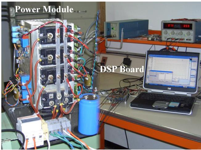
Figure 4: Experimental rig
