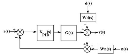
Figure 1: Control loop with a PID controller.
